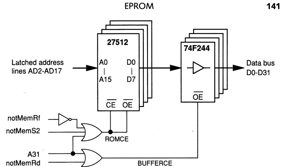
Figure 6.13 EPROM connection diagram showing output buffering.
