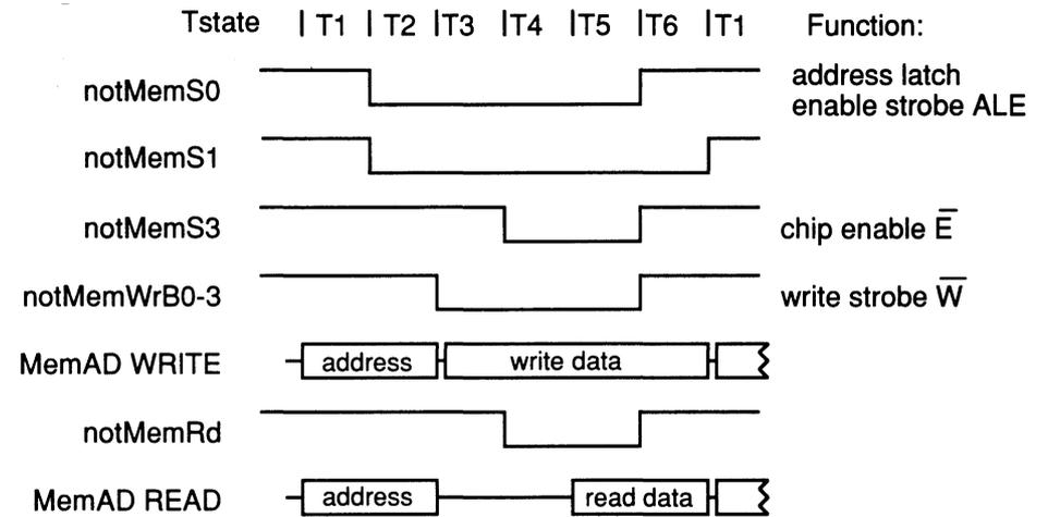
Figure 6.2 Internal configuration 8 for fast SRAM.
