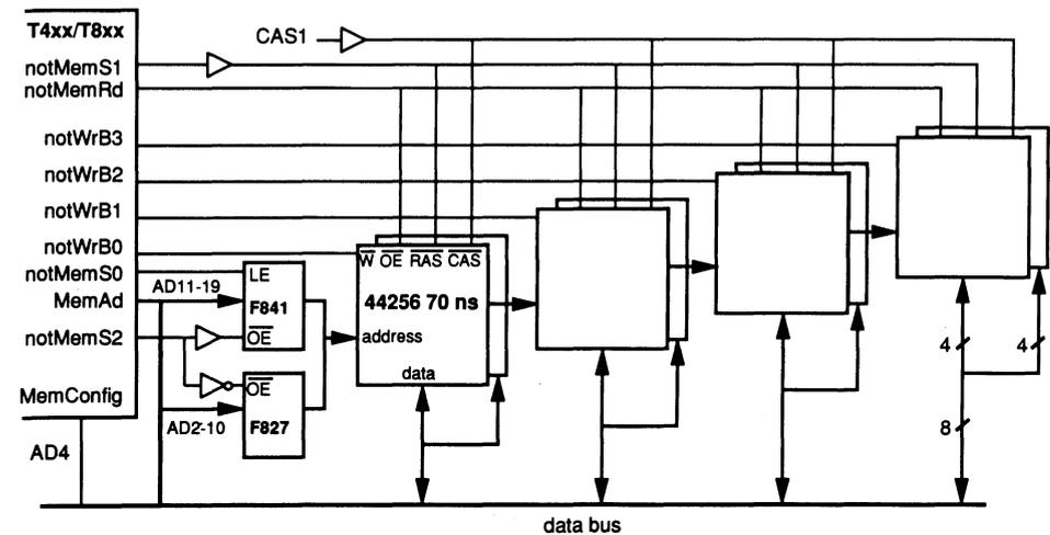
Figure 6.11 Memory connection diagram (only one bank shown).
