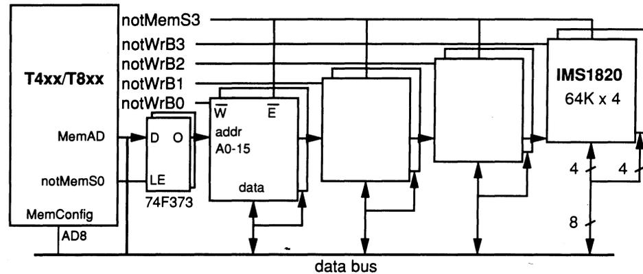
Figure 6.3 T4xx/T8xx with 256 kbytes of fast SRAM.
