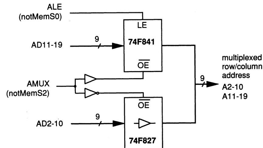
Figure 6.10 Row/column address multiplexer and address latch logic.
