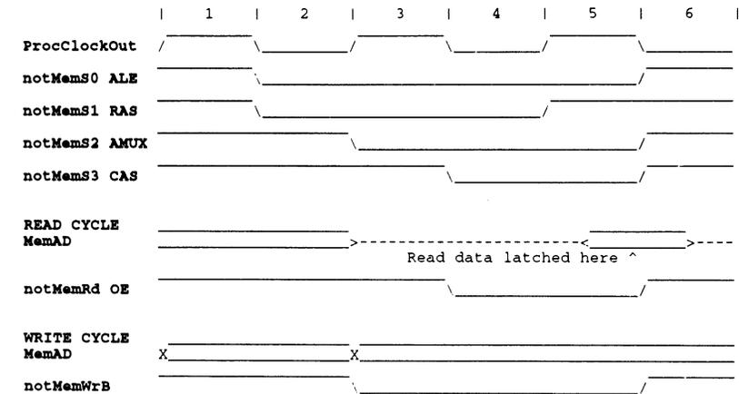
Figure 6.7 Timing diagram for DRAM running at zero wait states – configuration 4.
