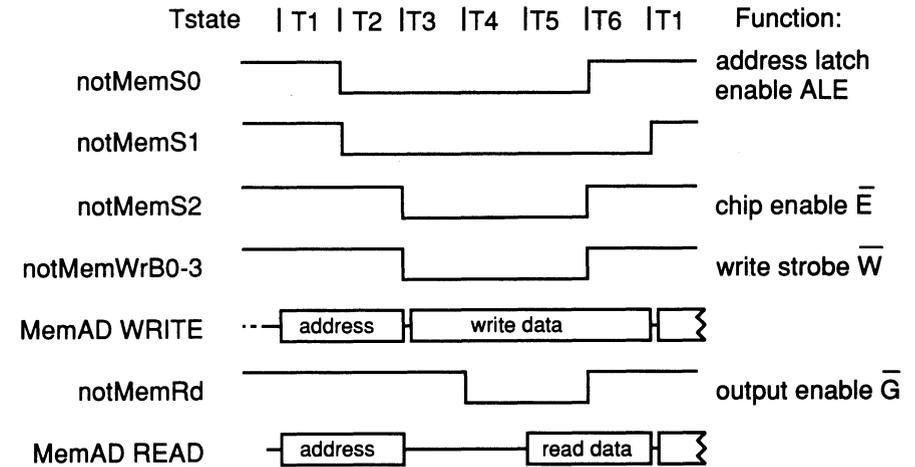
Figure 6.4 Modified strobe selection for SRAM with output enable.
