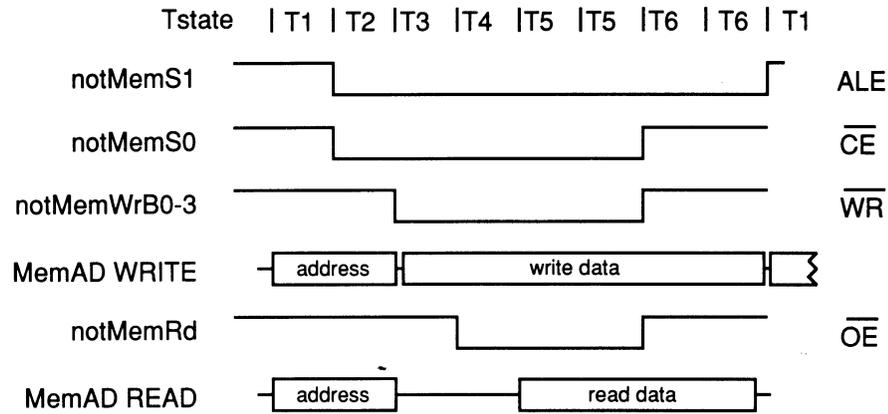
Figure 6.6 Timing configuration suitable for slower SRAM.
