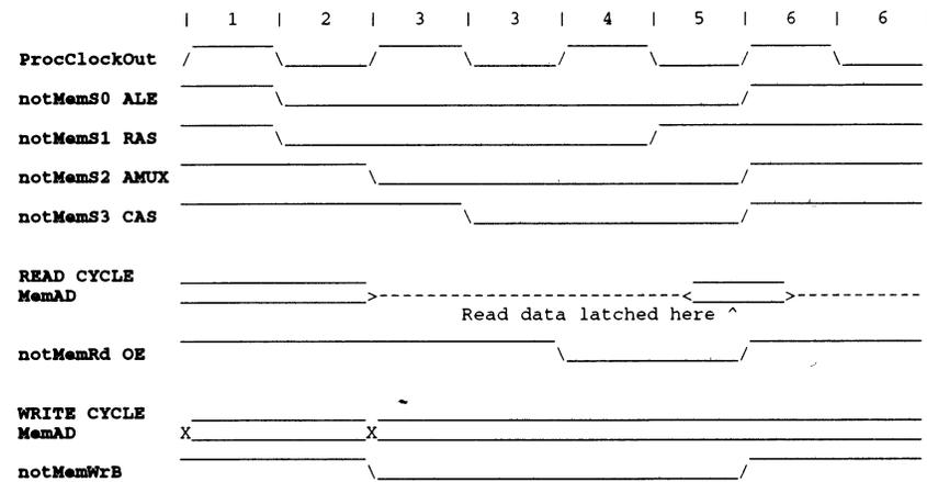
Figure 6.12 Four processor cycle memory configuration for 80 ns DRAM.
