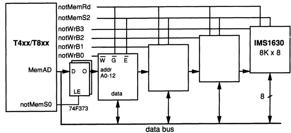
Figure 6.5 Connection of SRAM with output enable.
