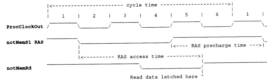
Figure 6.8 RAS access time and precharge time.
