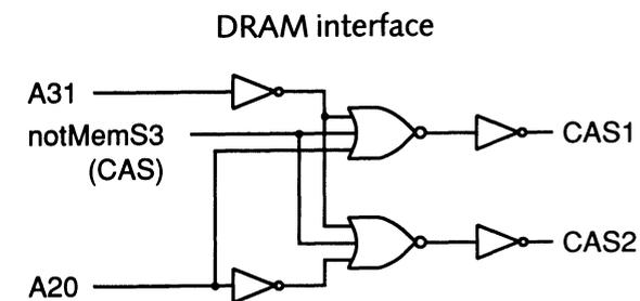
Figure 6.9 Column address strobe decoding logic.
