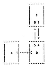
where each box represents a component; a line connecting two boxes represents a stream, with the arrow giving its direction, and number representing the file descriptor.
