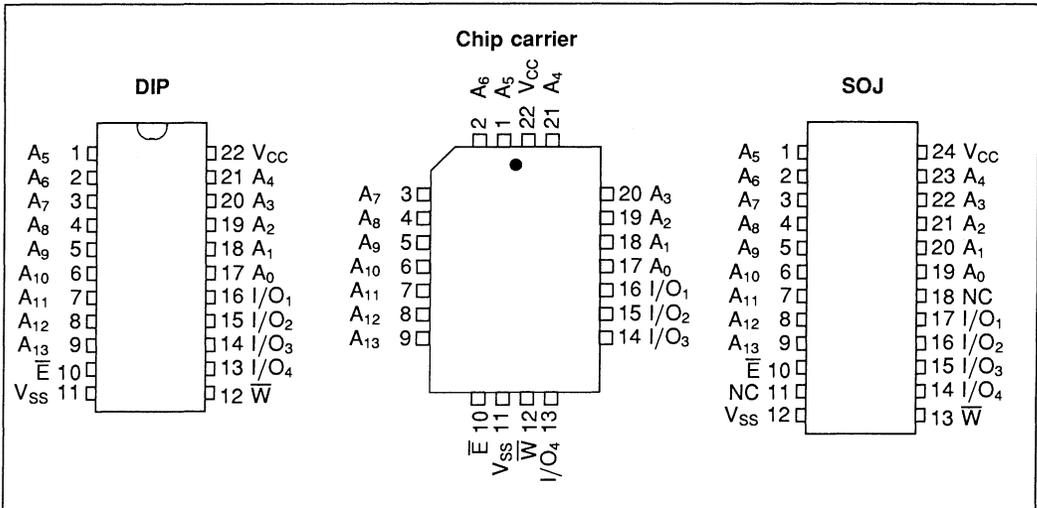
Figure 2.9 16K x 4 pin configuration
