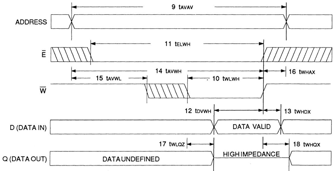
RECOMMENDED AC OPERATING CONDITIONS (-55°C ≤ T<sub>A</sub> ≤ +125°C) (V<sub>CC</sub> = 5.0V ±10%)
