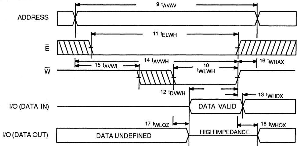
**RECOMMENDED AC OPERATING CONDITIONS** (-55°C ≤ TA ≤ 125°C) (Vcc = 5.0V ±10%)
