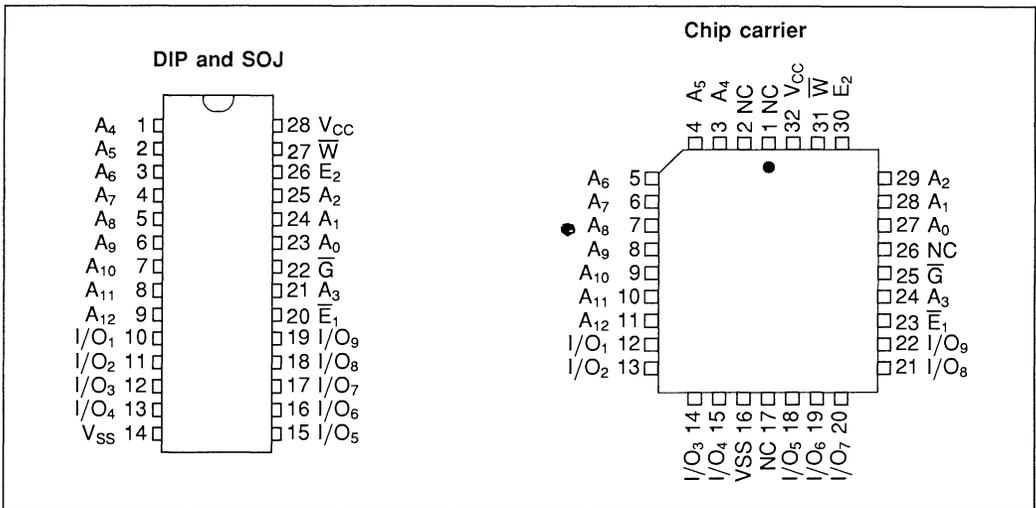
Figure 2.13 8K x 9 pin configuration
