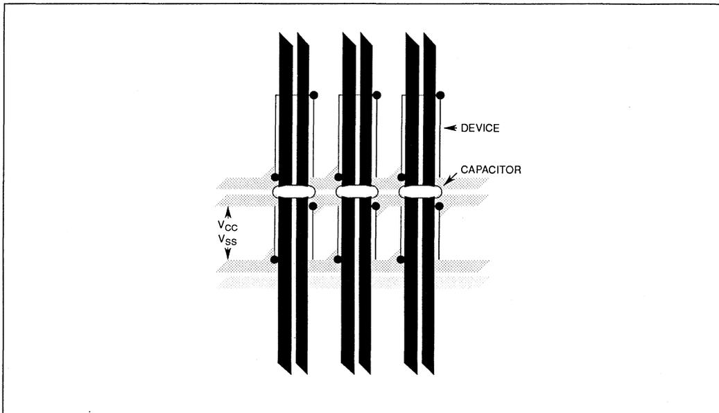
Figure 2.6 Grid showing decoupling capacitors
