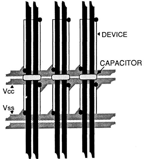
**$V_{CC}$ ,  $V_{SS}$  GRID SHOWING
