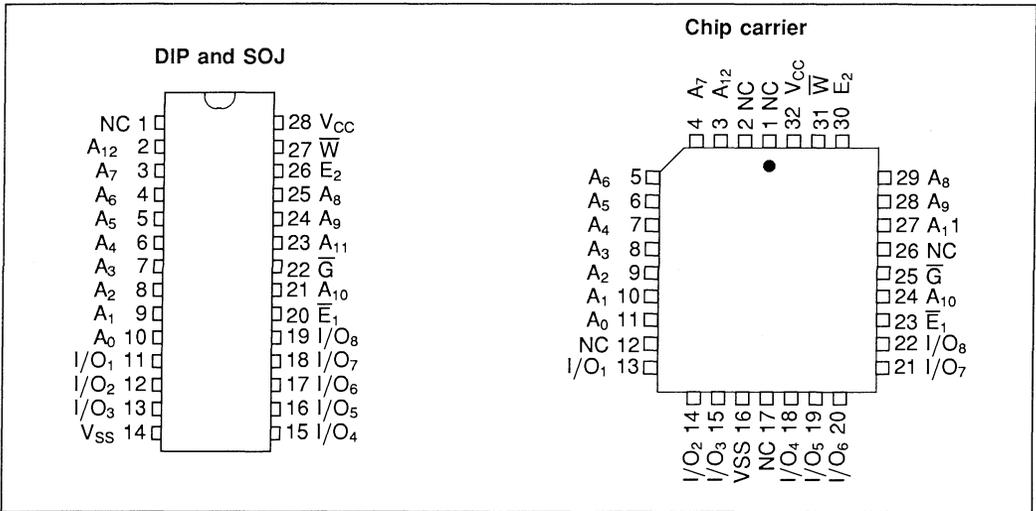
Figure 2.12 8K x 8 pin configuration
