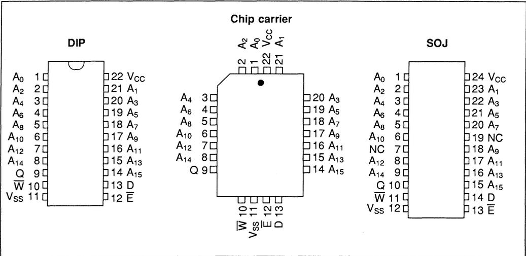
Figure 2.8 64K x 1 pin configuration
