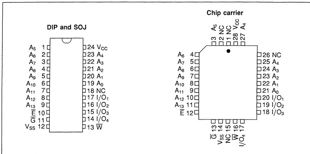
Figure 2.10 16K x 4 (with output enable) pin configuration
