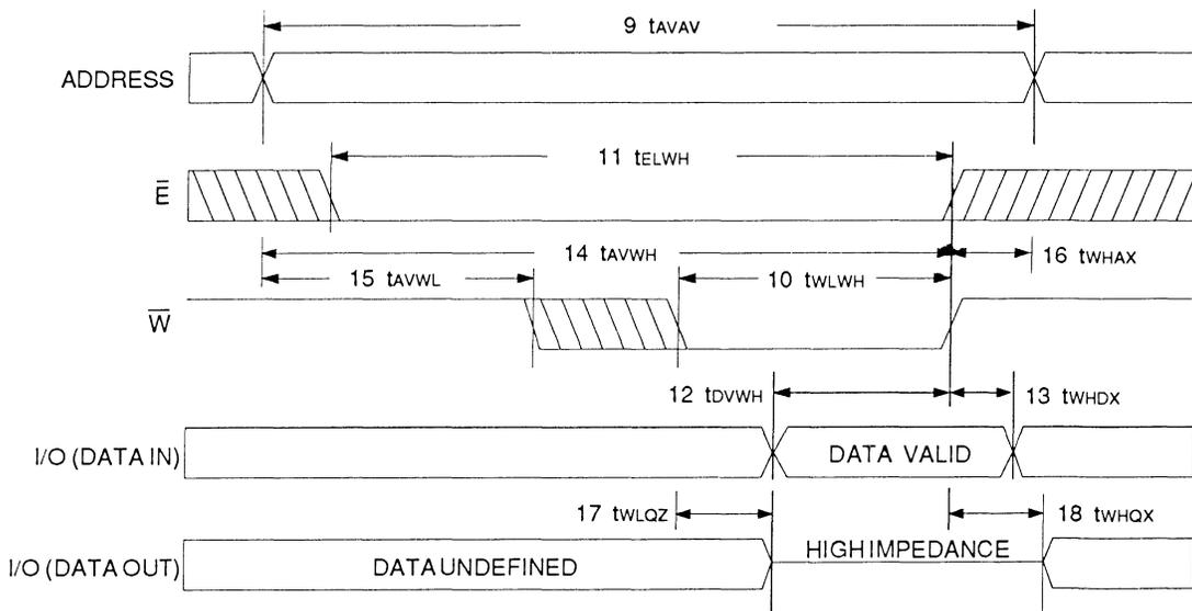
RECOMMENDED AC OPERATING CONDITIONS (-55°C ≤ Ta ≤ 125°C) (Vcc = 5.0V ±10%)
