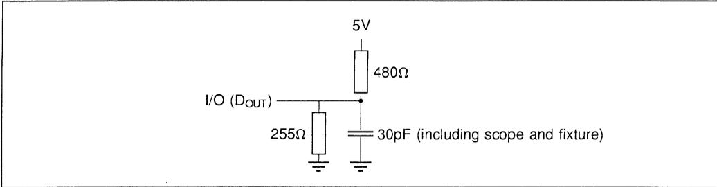
Figure 2.1 Output load
