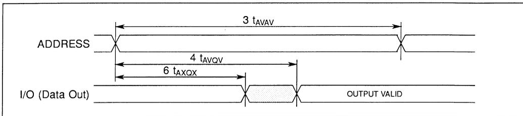
Figure 2.2 Read cycle 1<sup>a,d</sup>
