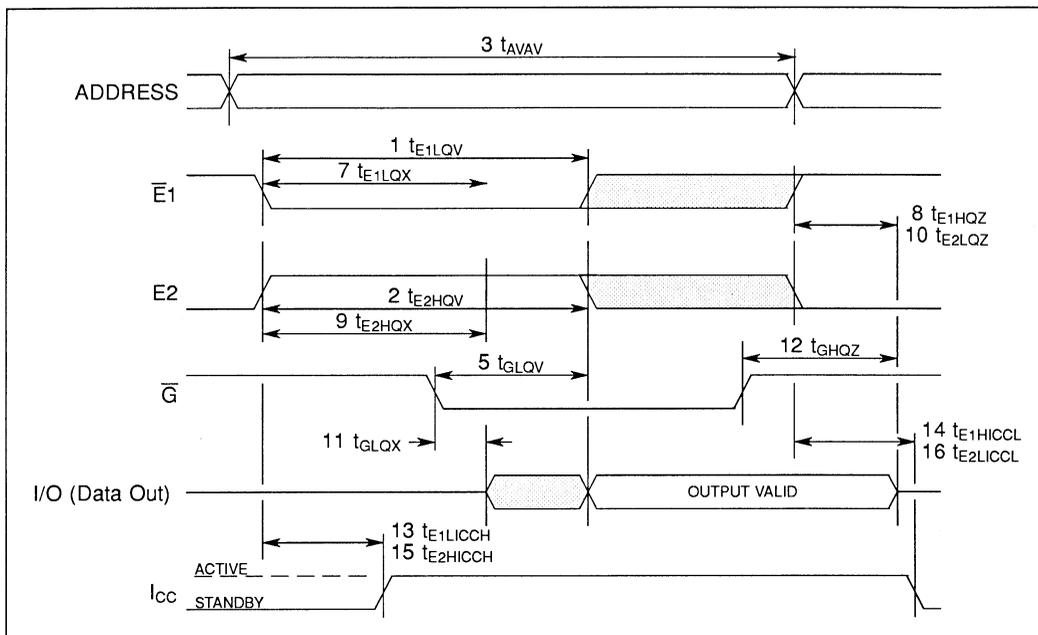
Figure 2.3 Read cycle 2<sup>c</sup>
