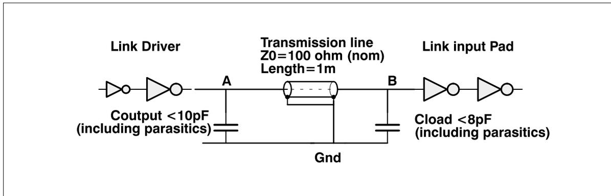
Figure C.1 Test Circuit
