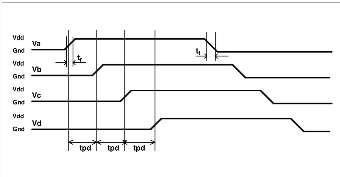
Figure D.2 Output Pad Timing
