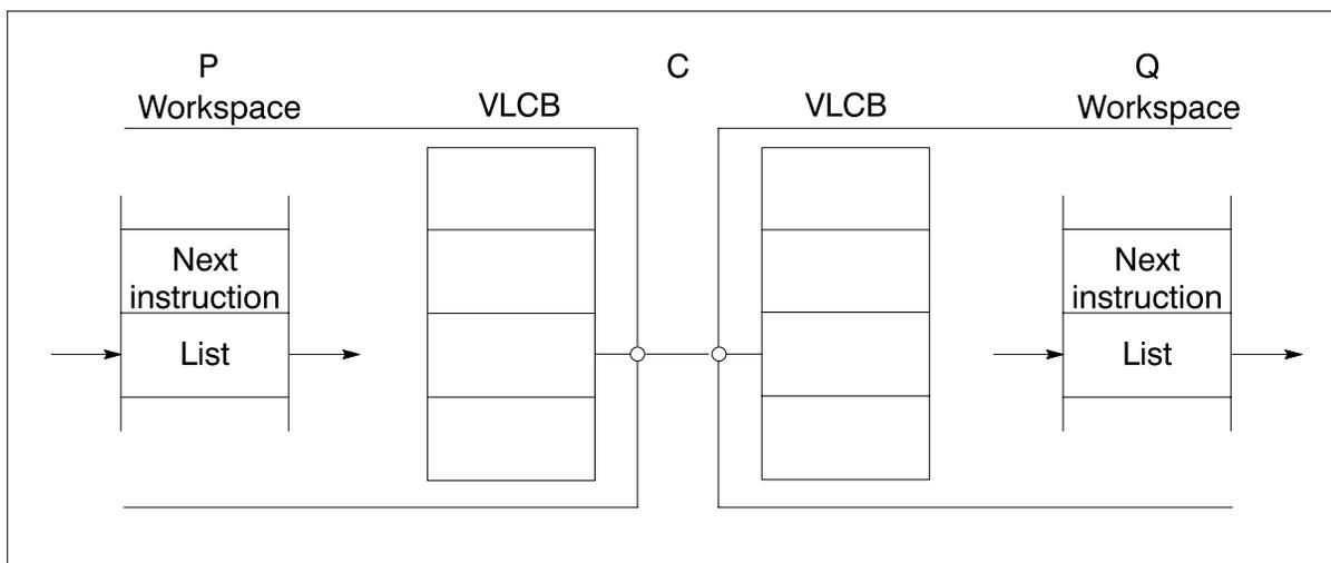
Figure 2.12 Communication completed
