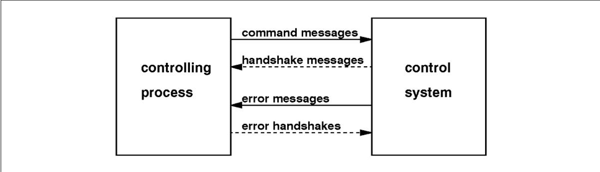
Figure 5.3 Communication between control process and control system
