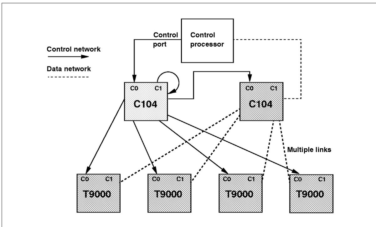
Figure 5.5 Routing control links through an IMS C104
