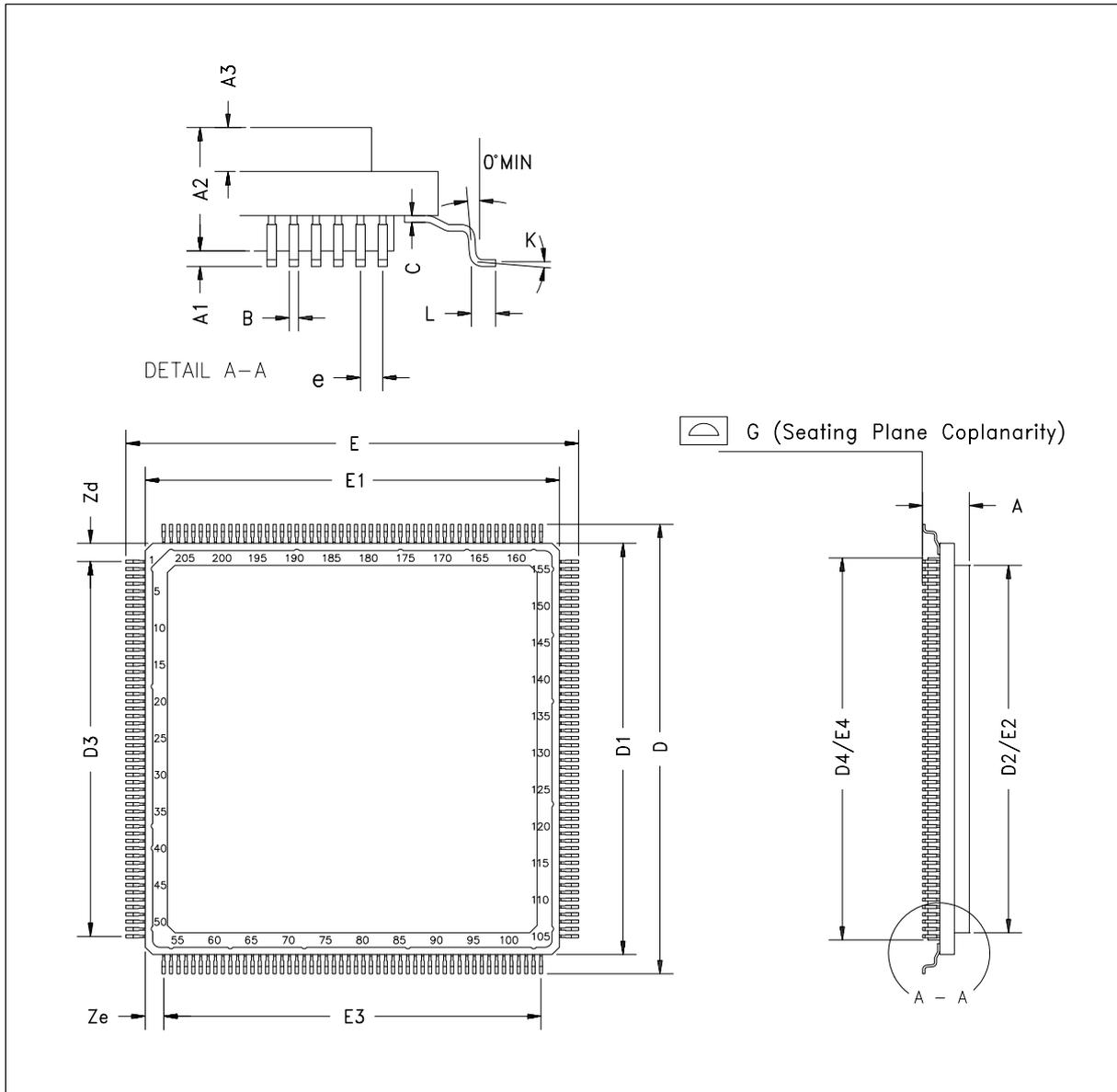
Figure 13.2 STC104 208 pin CLCC cavity-down package dimensions
