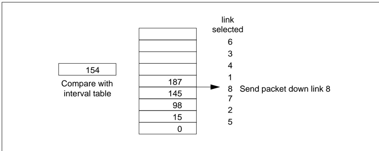
Figure 3.4 Interval labelling
