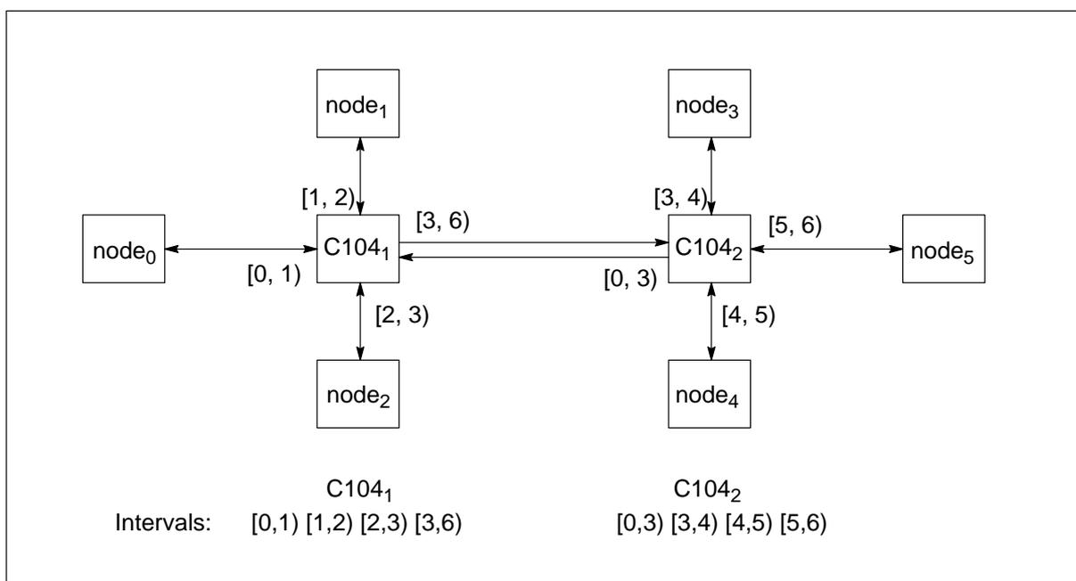
Figure 3.5 Interval routing
