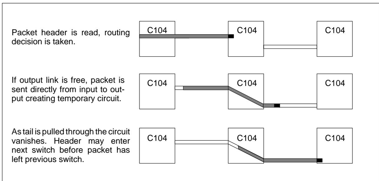
Figure 3.3 Wormhole routing
