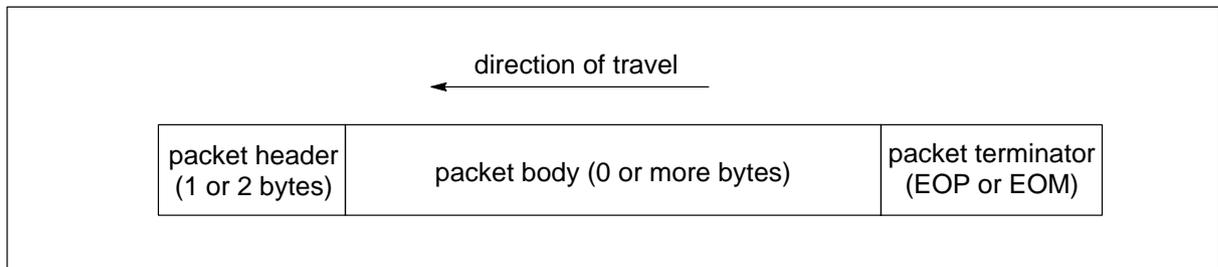
Figure 3.2 Packet structure
