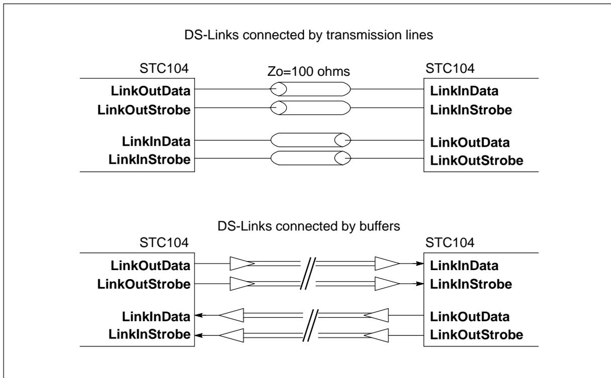
Figure 6.2 DS-Link connections
