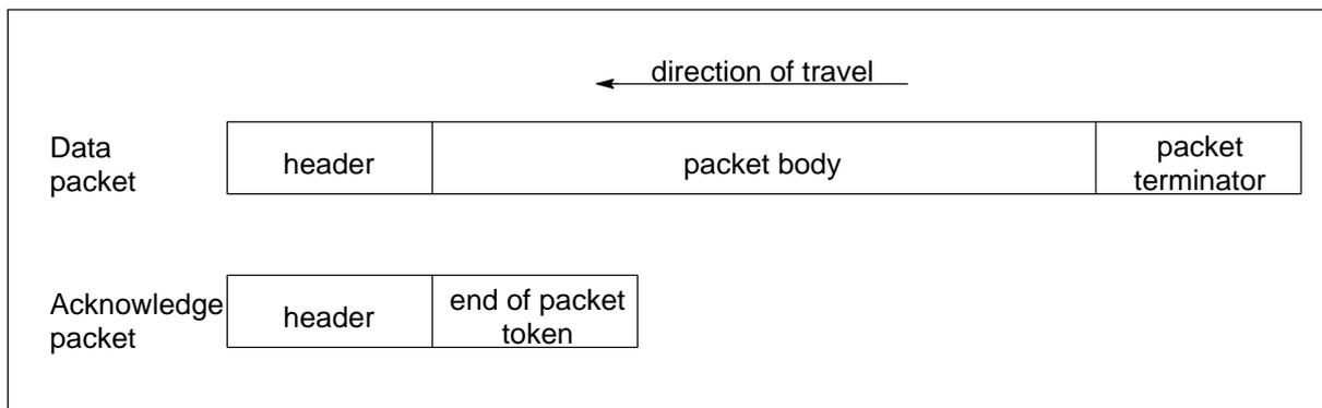
Figure 5.3 Structure of data and acknowledge packets
