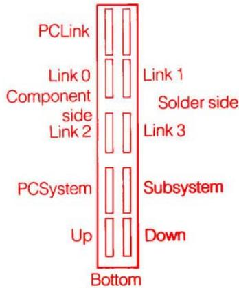
The diagram in the margin shows the rear edge connectors of the B004, looking from the rear of the board. As can be seen, there are two columns of pins, and these are grouped into sets of five, suitable for the five way sockets which terminate the various cables supplied.
