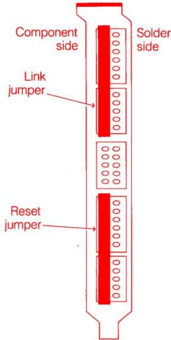
Before any program can be downloaded to a B004 board from a Personal Computer, two jumper sockets must be fitted correctly. The use of these jumpers allows more than one B004 to be present within a Personal Computer, but allowing only one of them to respond to the TDS. The board which has the jumpers fitted is designated the Master and any number of other INMOS evaluation boards can be attached to this one via the links.
