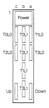
The B003 uses an edge connector pinout compatible with other INMOS transputer evaluation boards. The pinout is described in detail later in the user manual, but the figure in the margin shows what you need to know to connect to another board. The pins are grouped in sets of five, suitable for the five way sockets which terminate the various cables which plug into the edge connector. Each five way socket is coded to make it difficult to connect it to the wrong pins.
