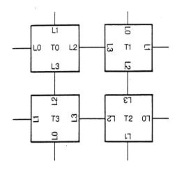
The IMS B003 evaluation board is a double extended Eurocard containing four T414 transputers, each with 256 Kbytes of dynamic RAM.
