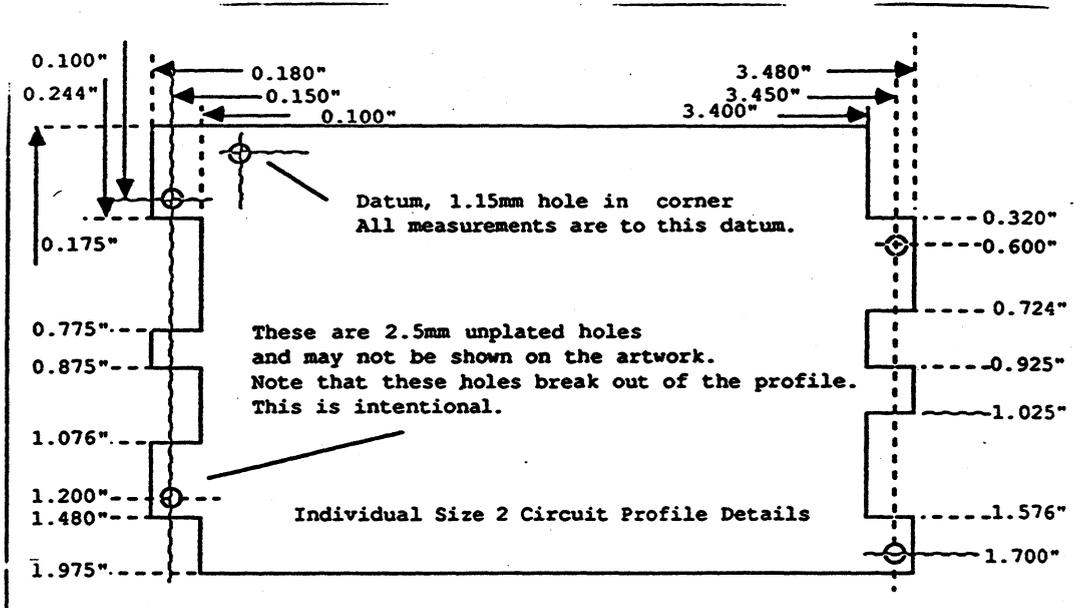
This tooling hole is 0.200" from the right edge and 0.150" from the top edge of the panel.
