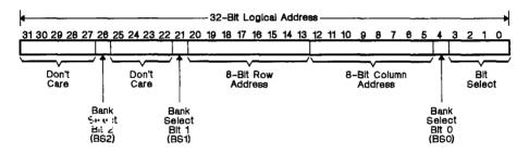
Figure 11-20. Address Decode for Example System
