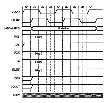
Figure 11-9. Local Bus Internal Cycles Back to Back
