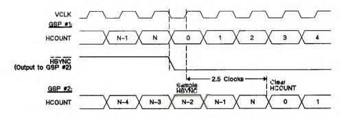
Figure 9-11. External Sync Timing - Two GSP Chips
