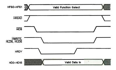
Figure 10-8. Host Interface Timing - Write Cycle With Wait
