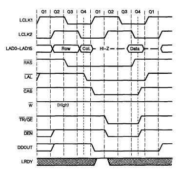
Figure 11-4. Local Bus Read Cycle Timing
