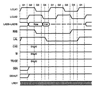
Figure 11-10. I/O Register Read Cycle Timing
