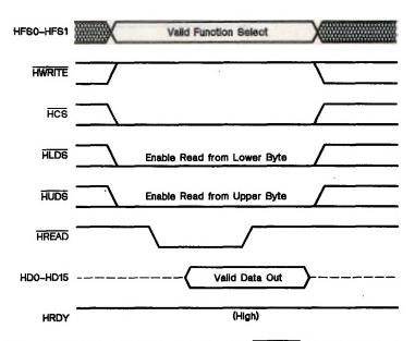
Figure 10-4. Host 16-Bit Read with HREAD Used as Strobe
