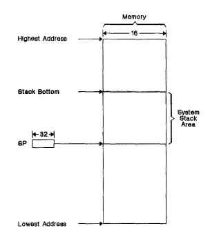
Figure 3-4. System Stack
