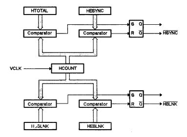
Figure 9-3. Horizontal Timing Logic - Equivalent Circuit
