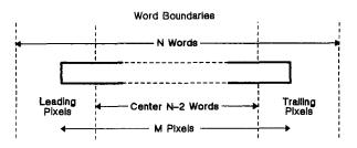
Figure 13-3. Pixel Block Alignment in X
