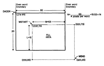
Figure 13-5. FILL XY Timing Example
