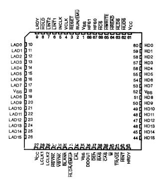
Figure 2-1. TMS34010 Pinout (Top View)
