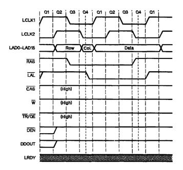
Figure 11-11. I/O Register Write Cycle Timing
