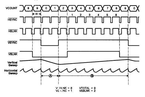
Figure 9-8. Noninterlaced Video Timing Waveform Example
