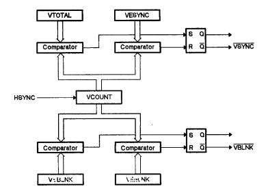
Figure 9-6. Vertical Timing Logic - Equivalent Circuit
