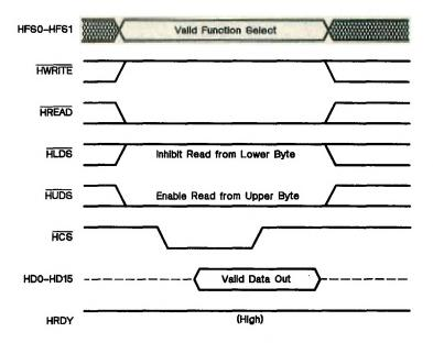
Figure 10-3. Host 8-Bit Read with HCS Used as Strobe
