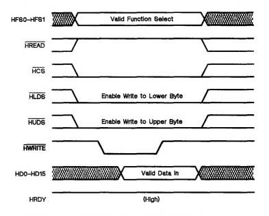
Figure 10-5. Host 16-Bit Write with HWRITE Used as Strobe
