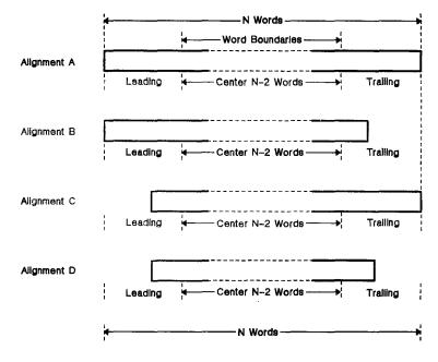
Figure 13-7. Pixel Block Alignments
