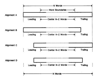
Figure 13-4. Pixel Block Alignments
