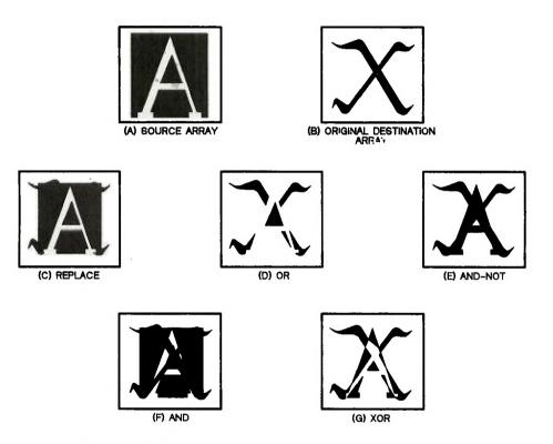
Figure 7-7. Examples of Operations on Single-Bit Pixels
