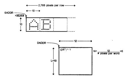
Figure 13-12. PIXBLT B,XY Timing Example
