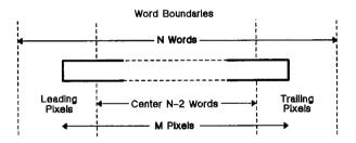
Figure 13-6. Pixel Block Alignment in X
