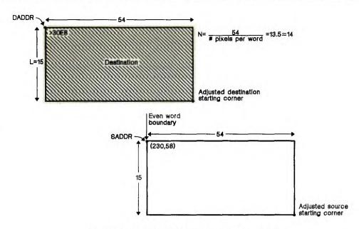
Figure 13-9. PIXBLT XY,L Timing Example
