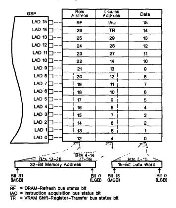
Figure 11-1. Triple Multiplexing of Addresses and Data
