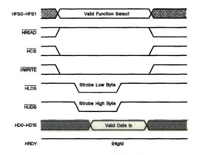
Figure 10-6. Host 16-Bit Write with HLDS, HUDS Used as Strobes
