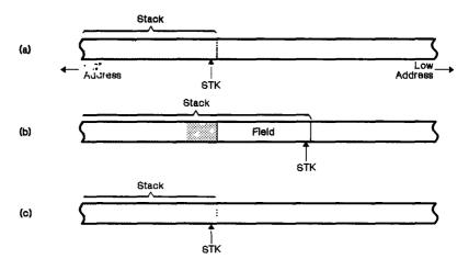
Figure 3-6. Auxiliary Stack Grows toward Lower Addresses
