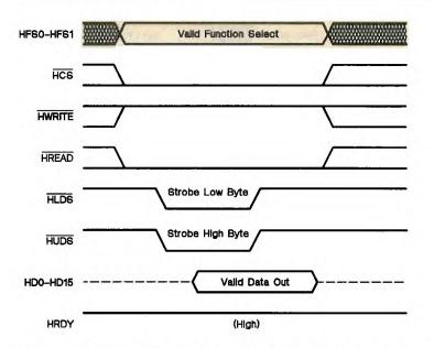
Figure 10-7. Host 16-Bit Read with HLDS, HUDS Used as Strobes
