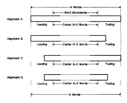
Figure 13-11. Pixel Block Row Alignments
