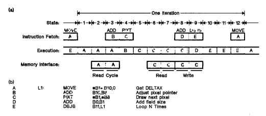
Figure 5-9. Parallel Operation of Cache, Execution Unit, and Memory Interface
