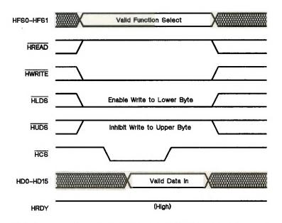
Figure 10-2. Host 8-Bit Write with HCS Used as Strobe
