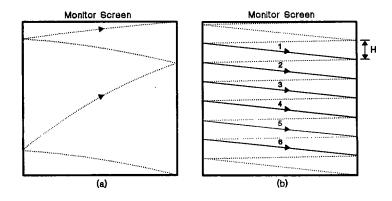
Figure 9-7. Electron Beam Pattern for Noninterlaced Video
