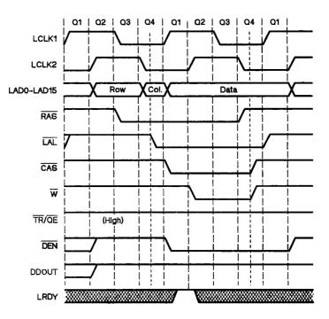
Figure 11-3. Local Bus Write Cycle Timing
