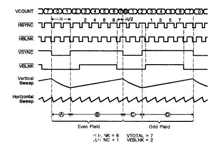
Figure 9-10. Interlaced Video Timing Waveform Example
