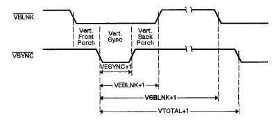
Figure 9-5. Vertical Timing for Noninterlaced Display
