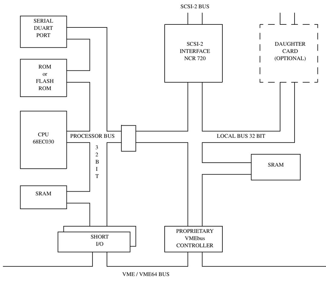
Figure 1-1. V/SCSI-2 Cougar II Block Diagram
