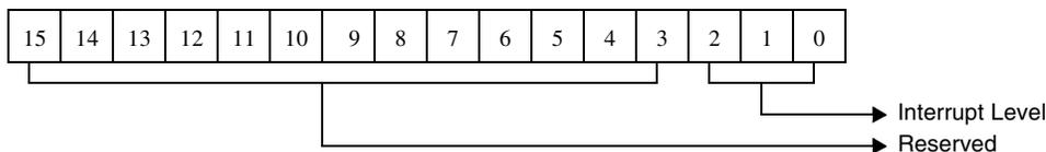
Figure 5-136. Interrupt Level For Download Firmware Command
