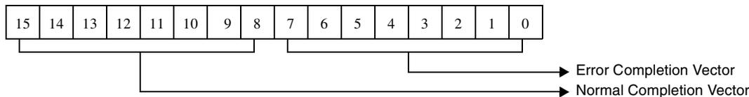
Figure 5-135. Normal/Error Completion For Download Firmware Command
