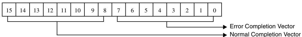
Figure 5-15. Normal/Error Completion Vector For SCSI Reset Command
