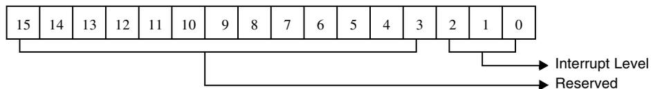
Figure 5-22. Interrupt Level For Printer Port Command
