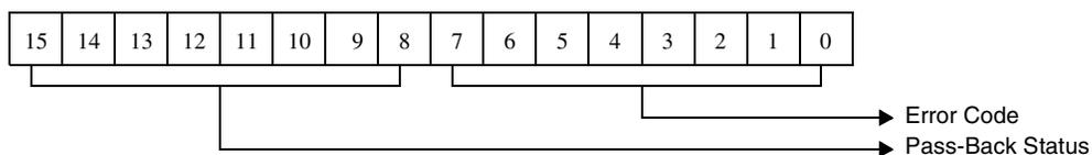
Figure 5-91. Return Status For Read/Write Buffer Command
