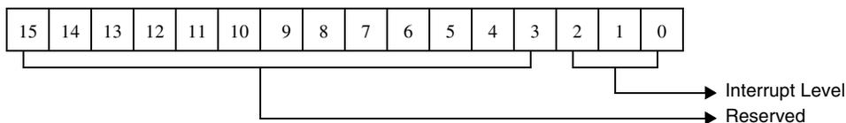
Figure 5-149. Interrupt Level For Buffer FIFO Command
