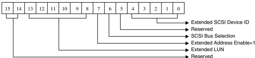
Figure 5-117. Extended Unit Address For Device Reinitialize Command
