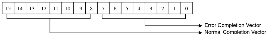
Figure 5-143. Normal/Error Completion Vector For Set Serial Number Command
