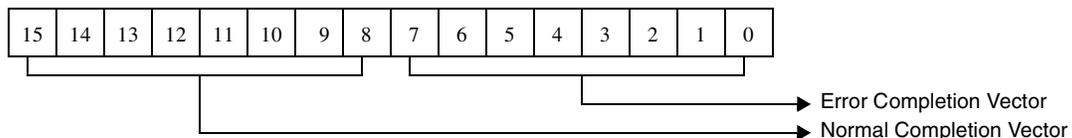
Figure 5-114. Normal/Error Completion Vector For Device Reinitialize Command
