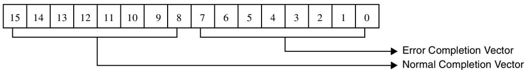
Figure 5-71. Normal/Error Completion For Dump Work Queue Parameters
