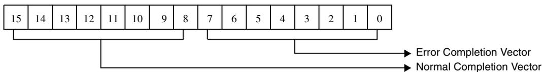
Figure 5-55. Normal/Error Completion Vector For Initialize Work Queue Command
