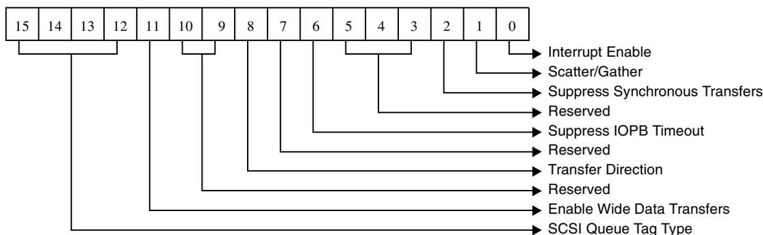
Figure 5-86. Command Options For Read/Write Buffer Command
