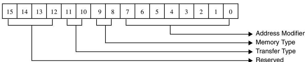
Figure 5-23. VME Transfer Types For Printer Port
