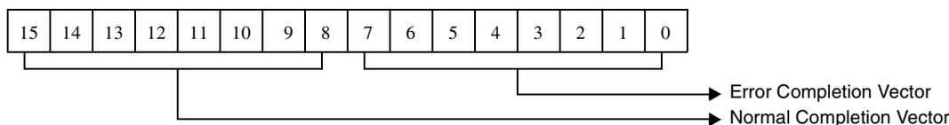
Figure 5-94. Normal/Error Completion Vector For Cancel Command Tag Command
