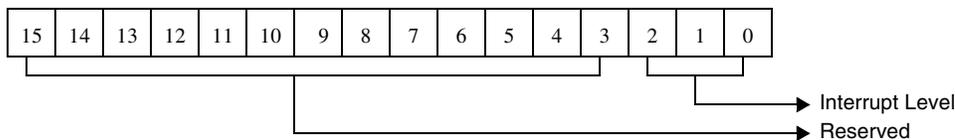
Figure 5-105. Interrupt Level For Initialize Printer Port Command
