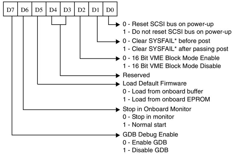
Figure 3-16. Software Configuration Jumper Settings Reported In Configuration Status Block
