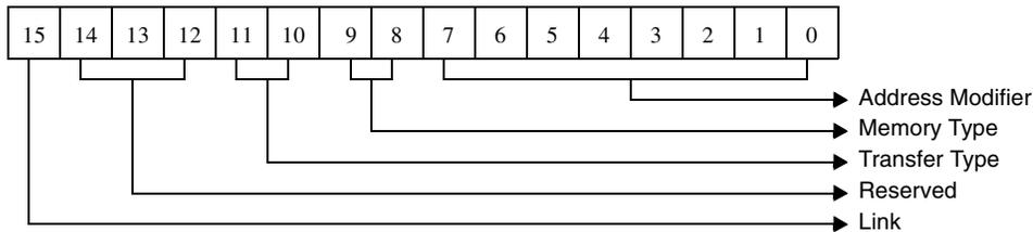
Figure 5-89. VME Transfer Types For Read/Write Buffer Command
