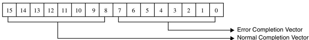
Figure 5-87. Normal/Error Completion Vector For Read/Write Buffer Command
