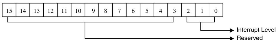
Figure 5-144. Interrupt Level For Set Serial Number Command
