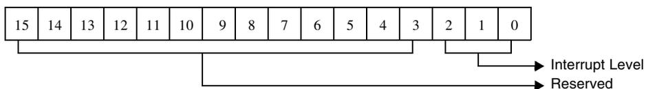
Figure 5-16. Interrupt Level For SCSI Reset Command
