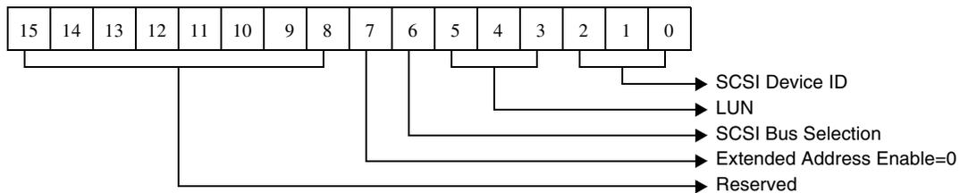
Figure 5-123. Unit Address For Issue Bus Device Reset Message Command
