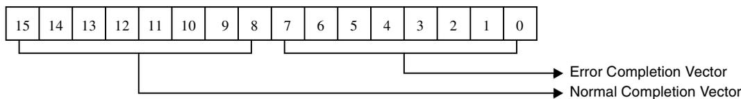
Figure 5-110. Normal/Error Completion for Restart Controller Command
