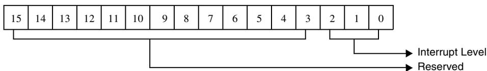
Figure 5-122. Interrupt Level For Issue Bus Reset Message Command
