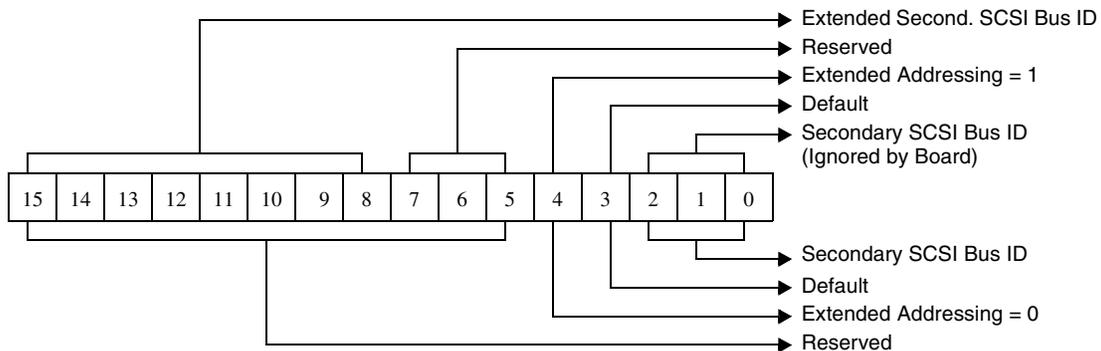
Figure 5-46. Secondary SCSI Bus ID For Controller Initialization Block
