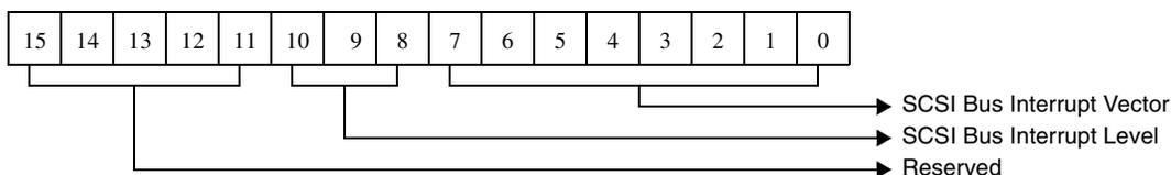
Figure 5-51. SCSI Bus Reset Interrupt Vector/Level for Controller Initialization Block
