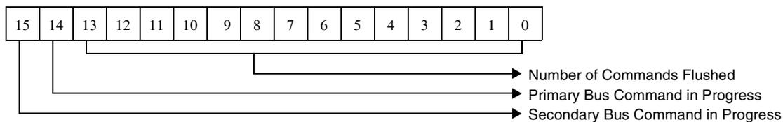
Figure 5-101. Commands Flushed In Progress Commands
