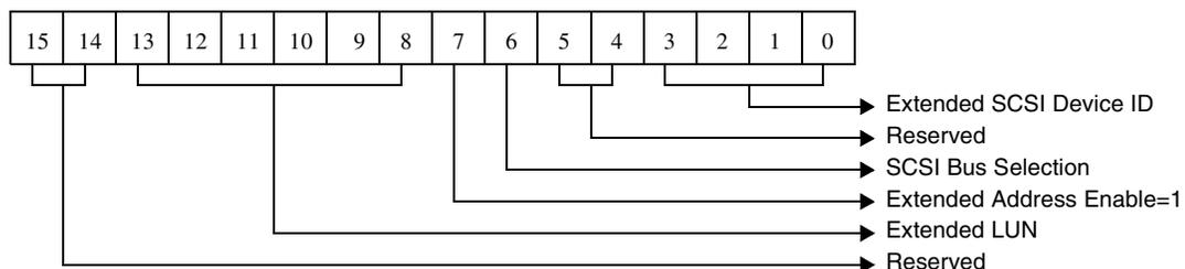
Figure 5-11. Extended Unit Address For SCSI Pass-Through Command
