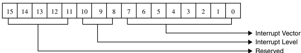
Figure 5-43. Controller Error Completion Level/Vector For Controller Initialization Block
