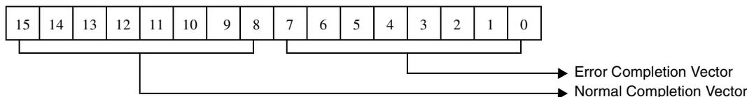
Figure 5-148. Normal/Error Completion Vector For Buffer FIFO Command
