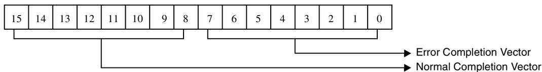
Figure 5-121. Normal/Error Completion For Issue Bus Device Message
