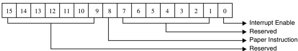
Figure 5-20. Command Options For Printer Port Command
