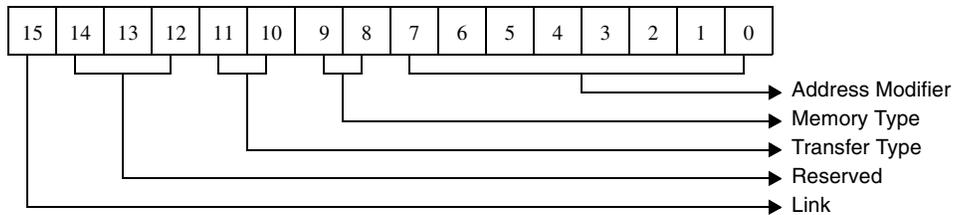
Figure 5-7. VME Transfer Types For SCSI Pass-Through Command
