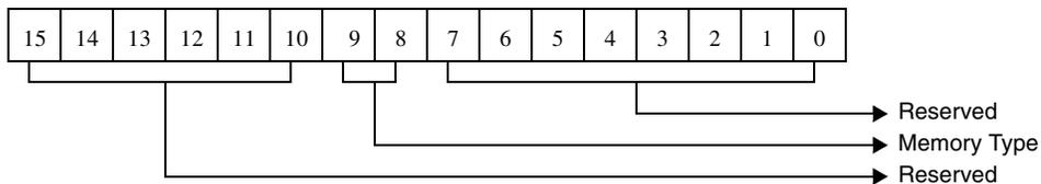
Figure 5-65. Memory/Transfer/Address Modifier For Dump Initialization Parameters Command
