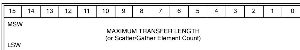
Figure 5-151. Maximum Transfer Length For Buffer FIFO Command
