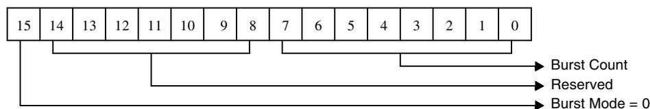
Figure 5-39. Burst Count Mode Enabled
