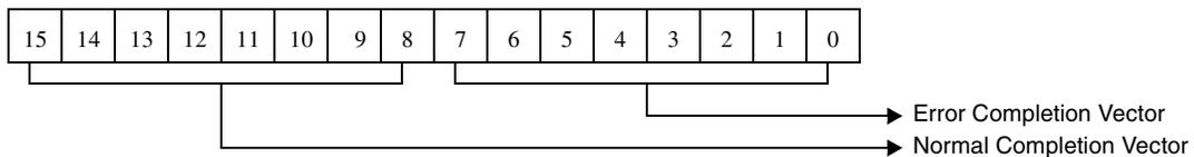
Figure 5-80. Normal/Error Completion Vector For Command Status Inquiry Command
