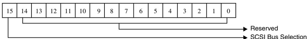
Figure 5-17. SCSI Bus ID For SCSI Reset Command
