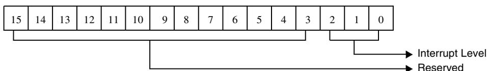
Figure 5-88. Interrupt Level For SCSI Pass-Through Command
