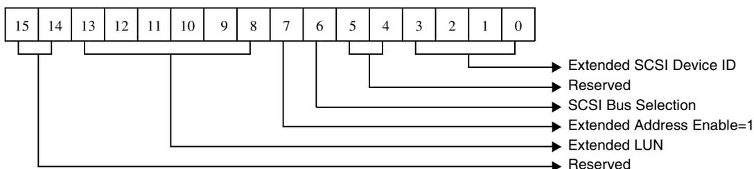
Figure 5-59. Extended Unit Address For Initialize Work Queue
