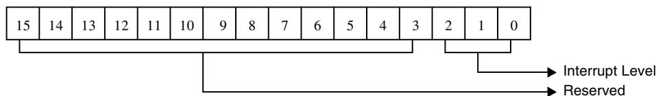
Figure 5-100. Interrupt Level For Flush Work Queue Command
