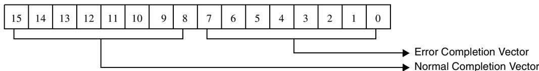
Figure 5-63. Normal/Error Completion Vector For Dump Initialization Parameters Commands
