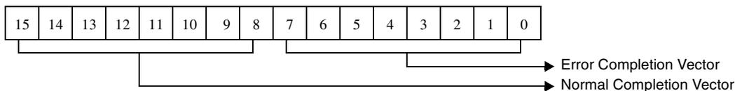
Figure 5-32. Normal/Error Completion Vector For Initialize Controller Command
