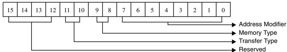
Figure 3-9. Memory Type/Transfer Type/Address Modifier
