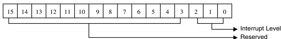
Figure 5-6. Interrupt Level For SCSI Pass-Through Command
