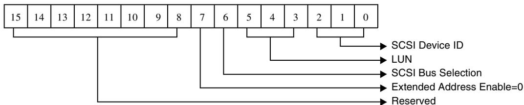
Figure 5-116. Unit Address For Device Reinitialize Command
