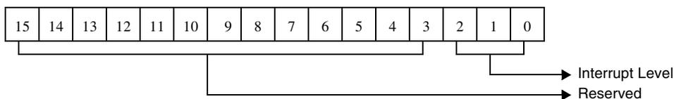
Figure 5-64. Interrupt Level For Dump Initialization Parameters Command
