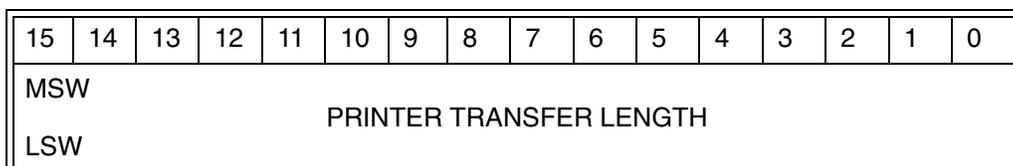
Figure 5-26. Printer Transfer Length For Printer Port Command
