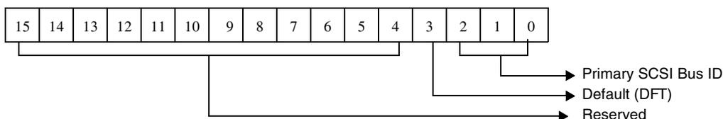
Figure 5-45. Primary SCSI Bus ID For Controller Initialization Block
