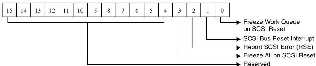
Figure 5-50. Error Recovery Options For Controller Initialization Block
