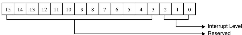
Figure 5-56. Interrupt Level For Initialize Work Queue Command
