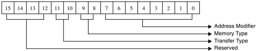
Figure 5-47. VME Transfer Type for Block Offboard Command Response
