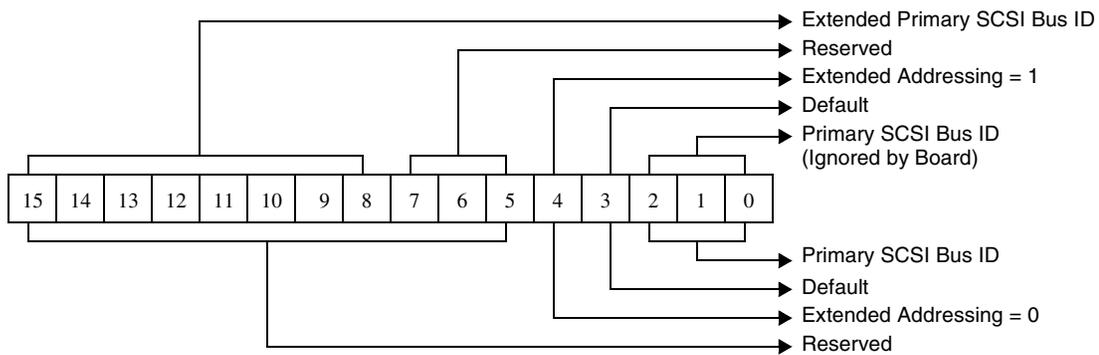
Figure 5-44. Primary SCSI Bus ID For Controller Initialization Block
