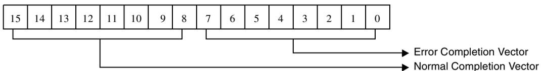
Figure 5-104. Normal/Error Completion Vector For Initialize Printer Port
