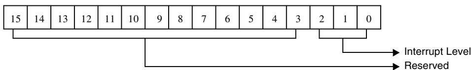
Figure 5-111. Interrupt Level For Restart Controller Command
