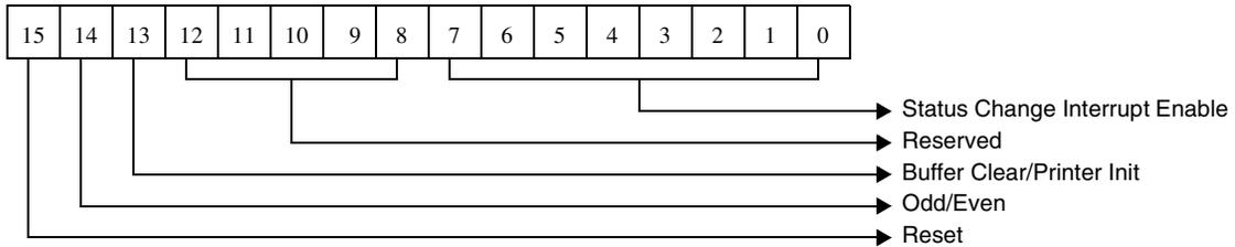
Figure 5-106. Printer Options For Initialize Printer Port Command
