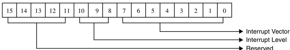
Figure 5-42. Controller Normal Completion Level/Vector For Controller Initialization Block
