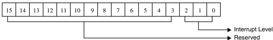
Figure 5-72. Interrupt Level For Dump Work Queue Parameters
