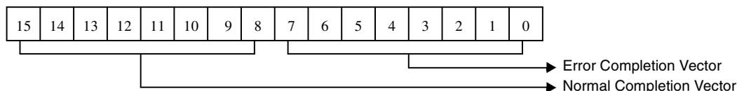
Figure 5-21. Normal/Error Completion Vector For Printer Port Command
