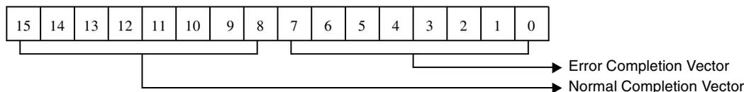
Figure 5-5. Normal/Error Completion Vector For SCSI Pass-Through Command
