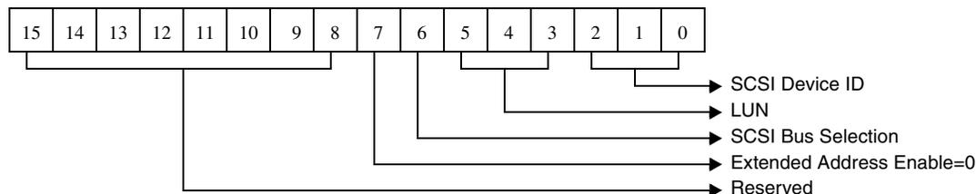
Figure 5-10. Unit Address For SCSI Pass-Through Command
