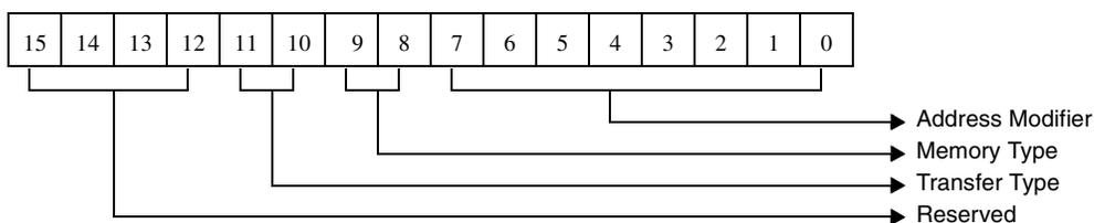
Figure 5-34. Address Modifier/Memory/Transfer Type For Initialize Controller Command
