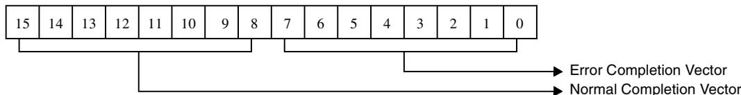
Figure 5-99. Normal/Error Completion Vector For Flush Work Queue Command
