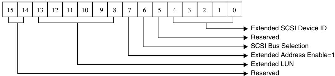
Figure 5-124. Extended Unit Address For SCSI Target Device
