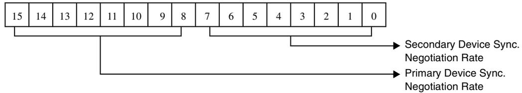
Figure 3-17. Synchronous Negotiation Rate
