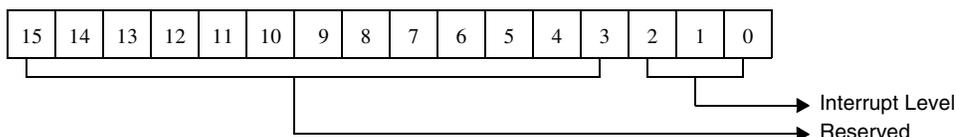
Figure 5-115. Interrupt Level For Device Reinitialize Command
