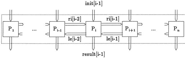
We assume that the sequence  $(x_1, x_2, \dots, x_n)$  to be sorted is available at channels  $\text{init}[0], \text{init}[1], \dots, \text{init}[n-1]$ . The sorted sequence may be outputed at channels  $\text{result}[0], \text{result}[1], \dots, \text{result}[n-1]$ . To describe the sorting process, we consider one process  $P_i$ . Let us suppose  $P_i$  is in an odd phase. The activities  $P_i$  has to execute depend on i:
