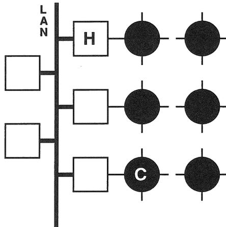
Figure 8: The General Multicomputer – Trolius is a uniform foundation for message passing on every multicomputer node. Host nodes (H) run Trolius with the local operating system while compute nodes (C) run it natively.
