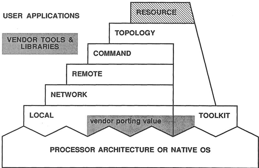
Figure 9: Trollius Layered Structure – Each layer has a standard interface accessible to the user. Vendors can add proprietary value in porting to specific hardware and in bundling tools and libraries. The resource layer is part of the third generation of Trollius.
