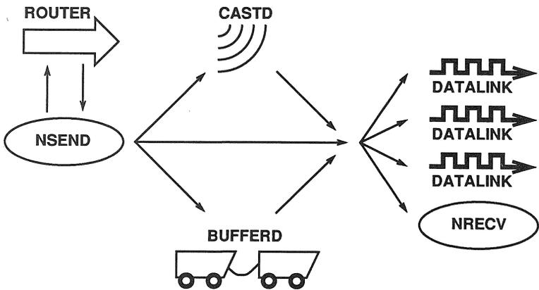
Figure 11: Network Forwarding Processes – After consulting the router, a process calling *nsend()* transfers the message to a local forwarding process. *Bufferd* can hold multiple messages, up to a space limit tuned by the user.
