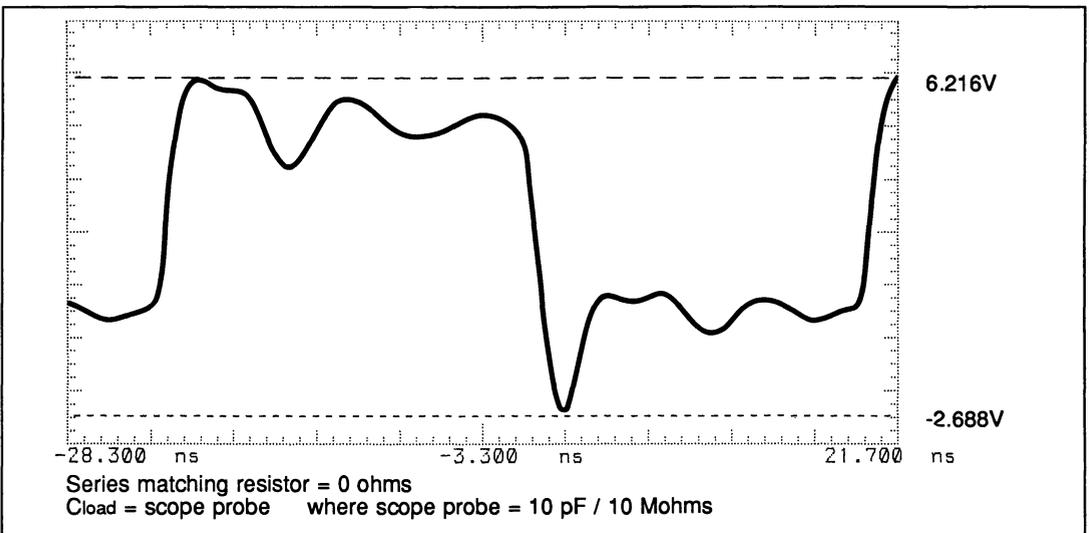
Figure 3.21 Under damped response (scope probe load)
