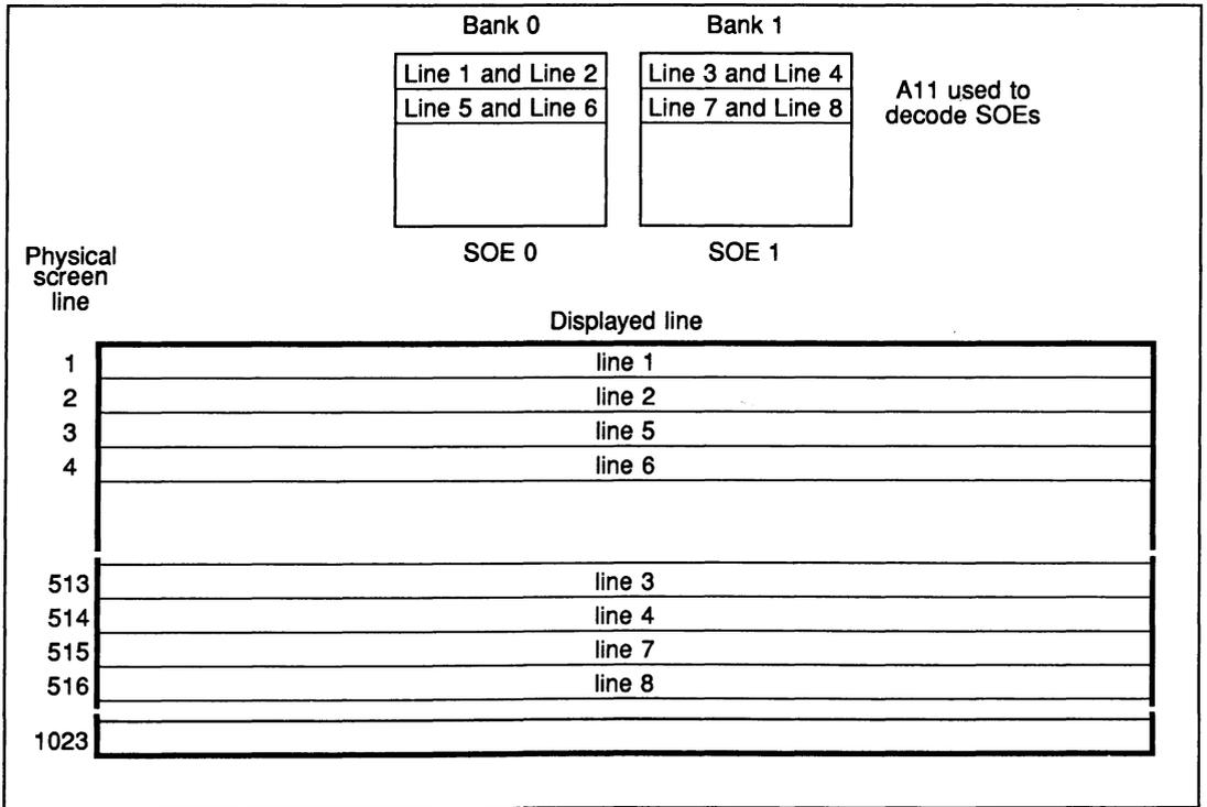
Figure 3.15 Effect of untransposed addresses on display
