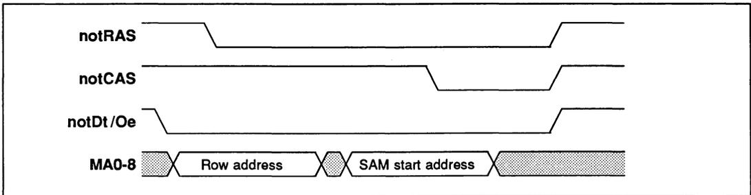
Figure 3.5 VRAM transfer timing
