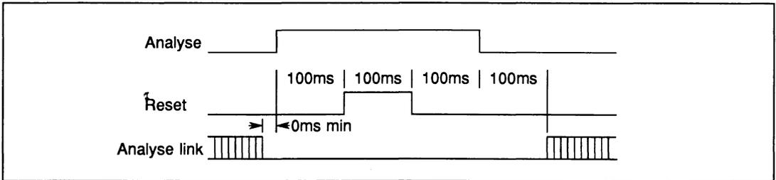
Figure A.5 Analyse timing
