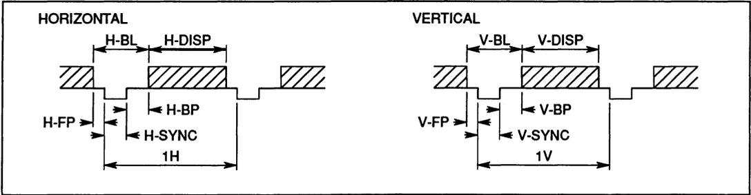
Figure A.1 Hitachi HM-4219/4119 timing
