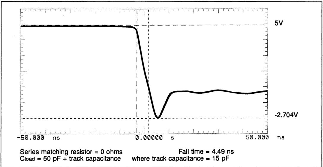
Figure 3.20 Under damped response
