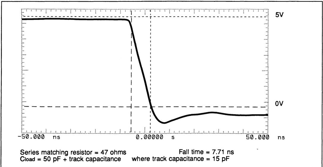
Figure 3.23 Optimally damped response
