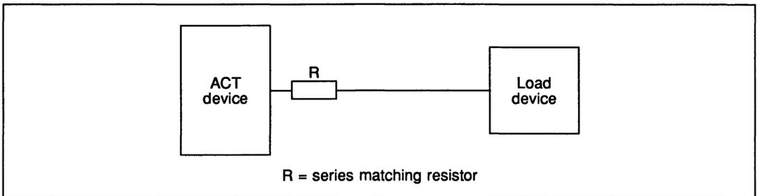
Figure 3.19 Test circuit for the effects of series matching resistor on damping
