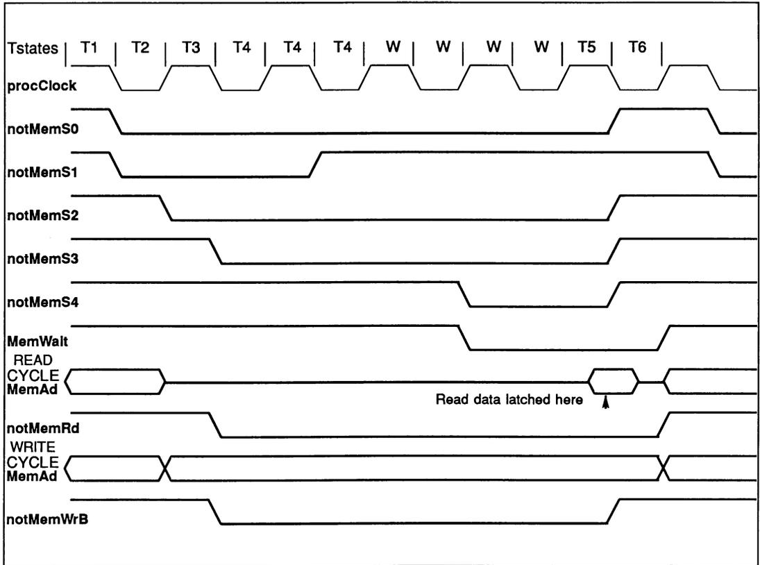
Figure A.3 Timing for extended memory cycle
