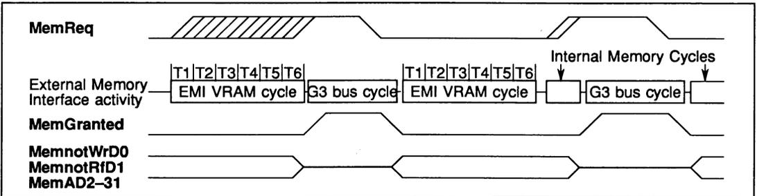
Figure 3.6 MemGranted with G3 bus cycles and external, internal memory cycles
