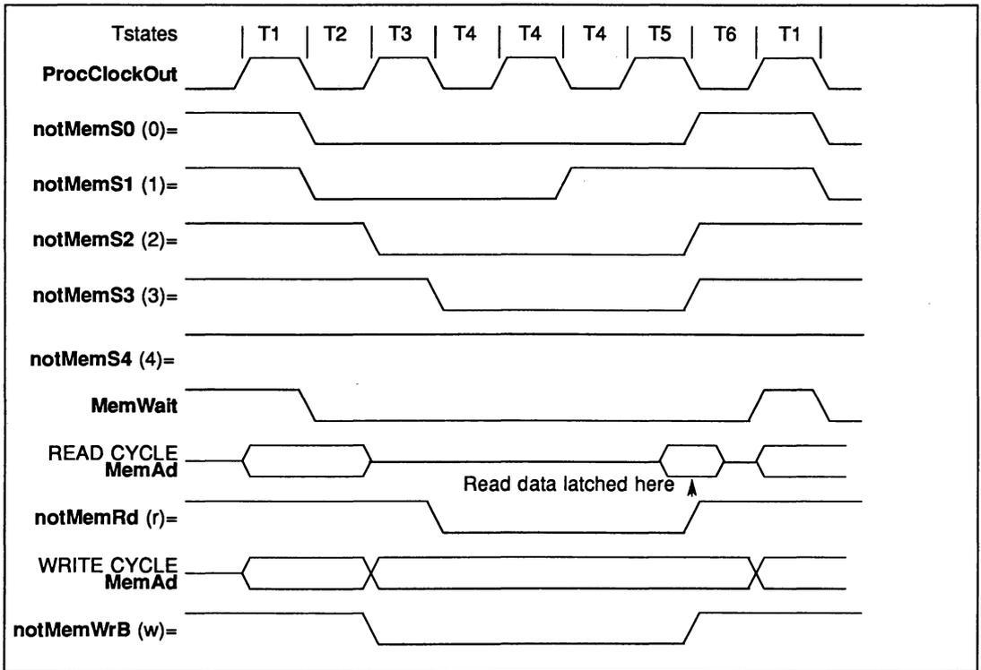
Figure 3.3 Timing for basic memory cycle
