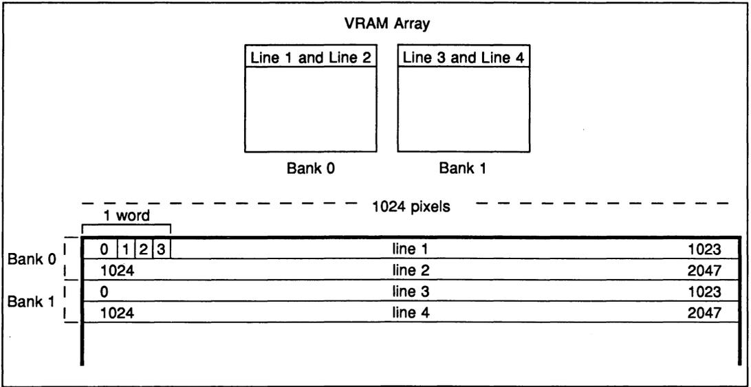
Figure 3.14 Example of 1024 x 1024 screen layout
