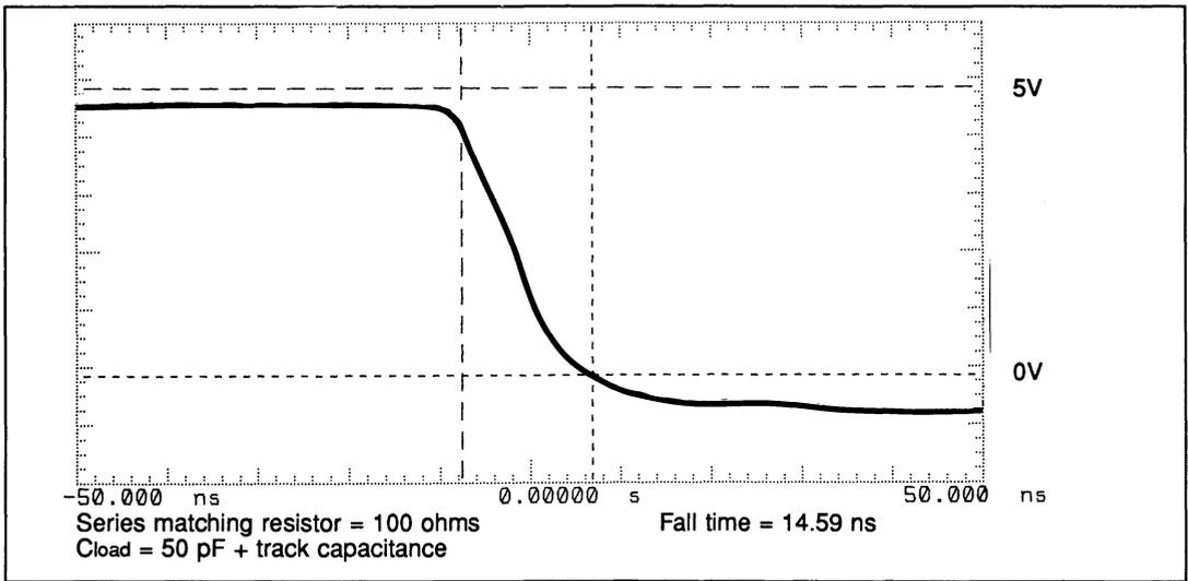
Figure 3.22 Over damped response
