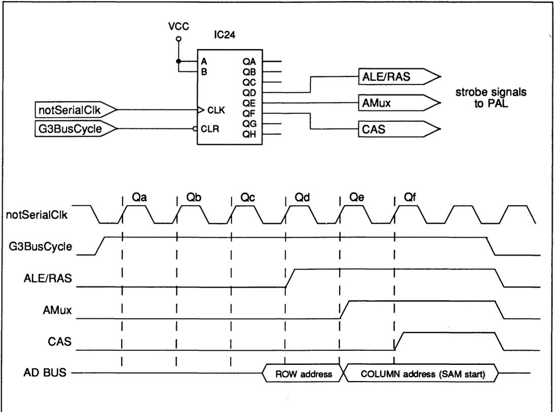
Figure 3.8 Memory strobe generation for G300 VRAM interface using a shift register
