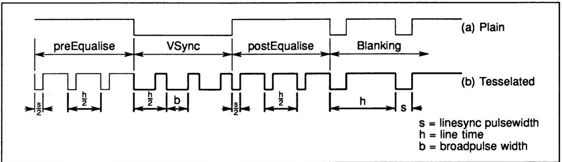
Figure 3.18 Composite sync frame flyback waveforms
