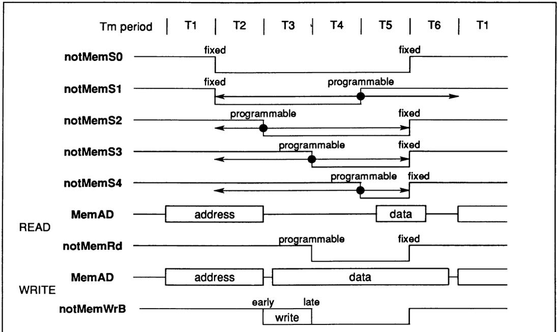
Figure 3.2 Generalised timing for EMI
