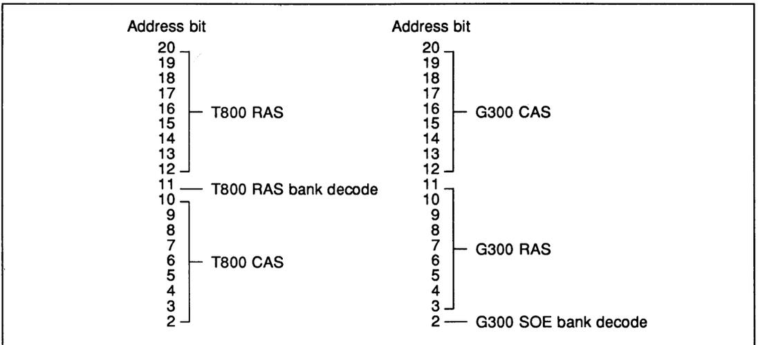
Figure 3.13 TRAM address multiplexing
