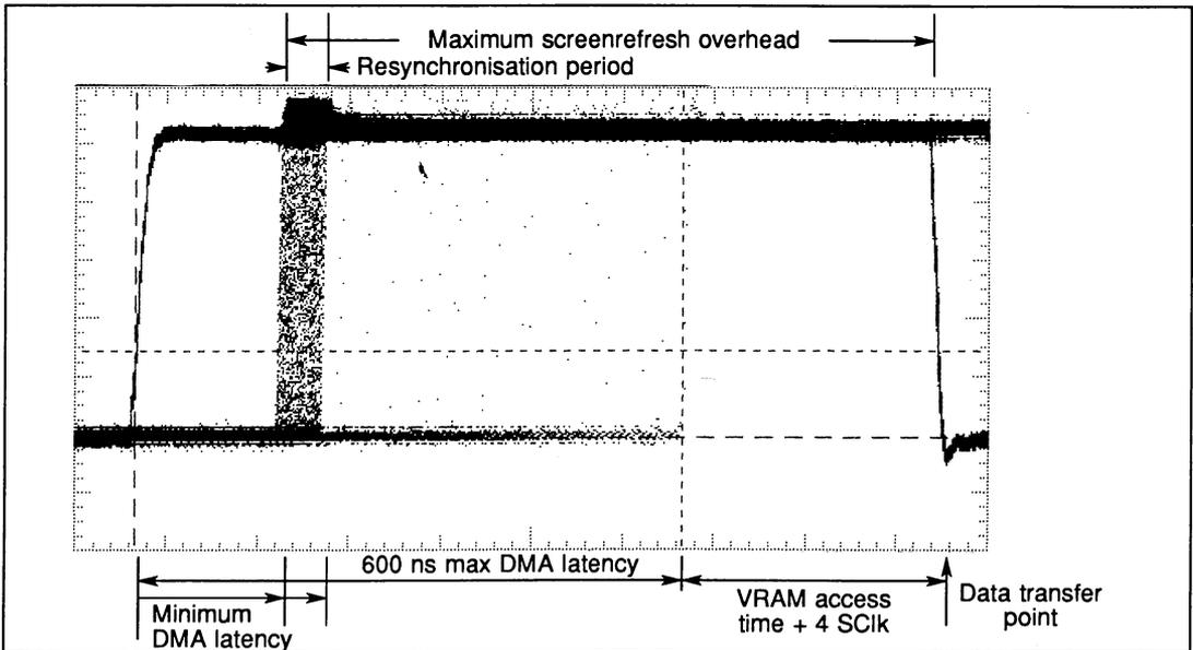
Figure 3.11 Measured DMA latency
