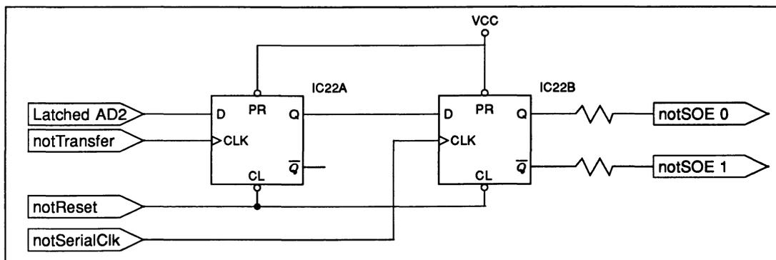
Figure 3.10 SOE decode
