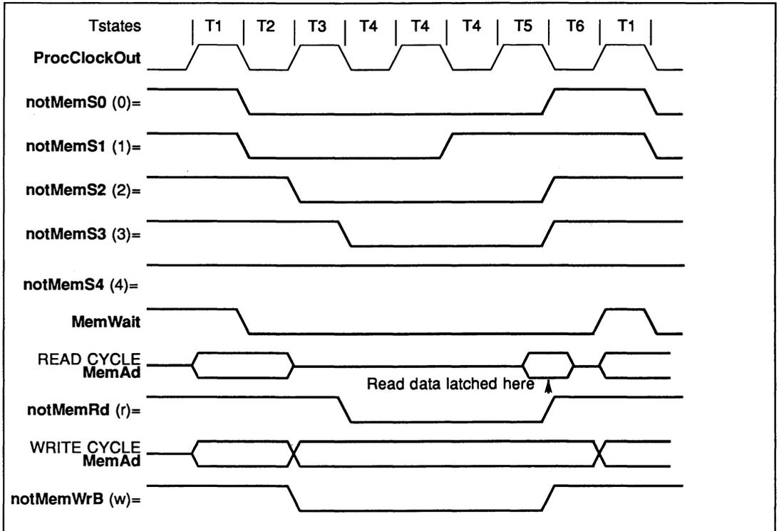
Figure A.2 Timing for basic memory cycle
