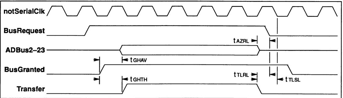
Figure 3.7 Data transfer timings for G300 CVC
