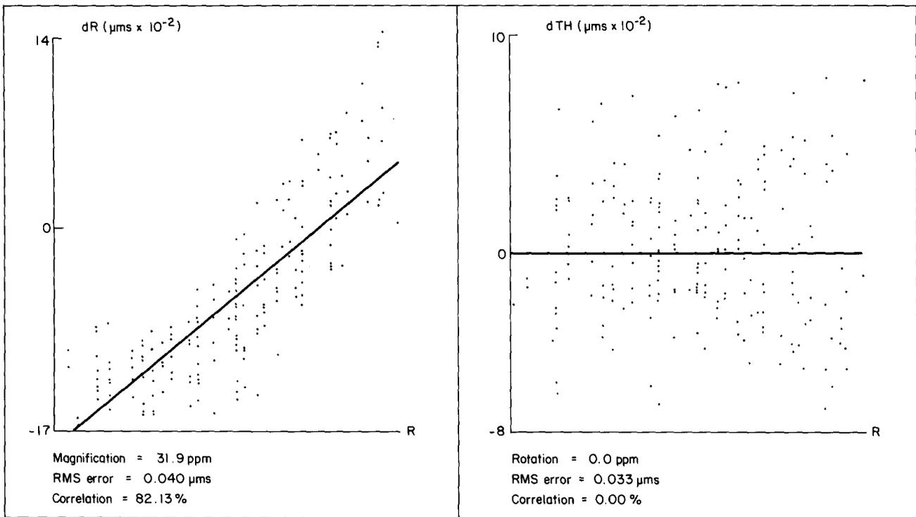
Fig 11 Polar errors showing rotation and reduction
