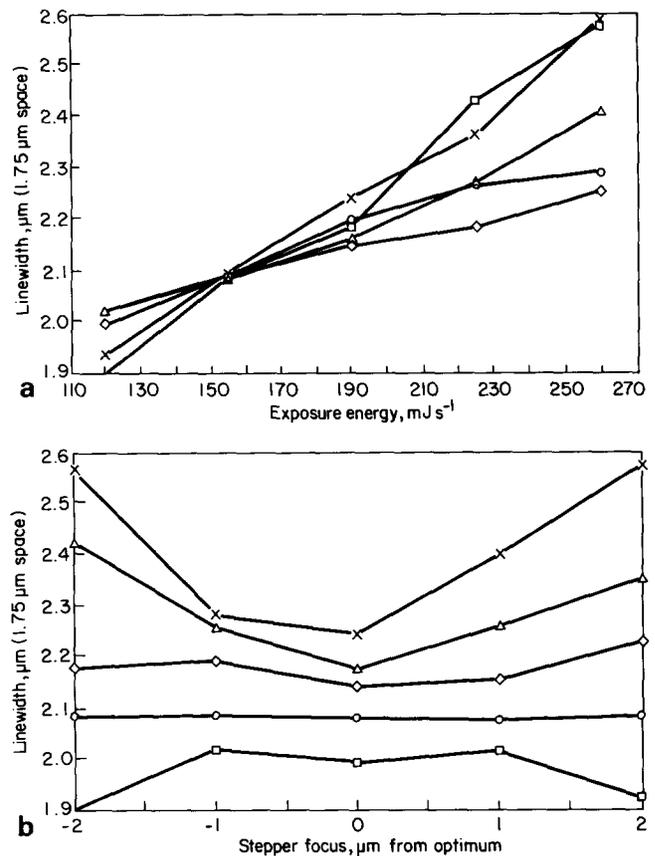
**Fig 3** Process characteristic graphs: (a) Inmos T800 photolithography, linewidth against exposure,  $\square$  = -2  $\mu\text{m}$ ,  $\circ$  = -1  $\mu\text{m}$ ,  $\diamond$  = optimum,  $\triangle$  = +1  $\mu\text{m}$ ,  $\times$  = +2  $\mu\text{m}$ ; (b) linewidth against focus,  $\square$  = 120 mJ,  $\circ$  = 155 mJ,  $\diamond$  = 190 mJ,  $\triangle$  = 225 mJ,  $\times$  = 260 mJ
