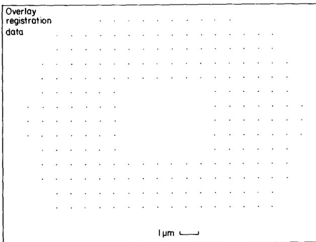
Fig 14 Overlay of first and second lenses to 0.18 µm specification. (All points are within specification)
