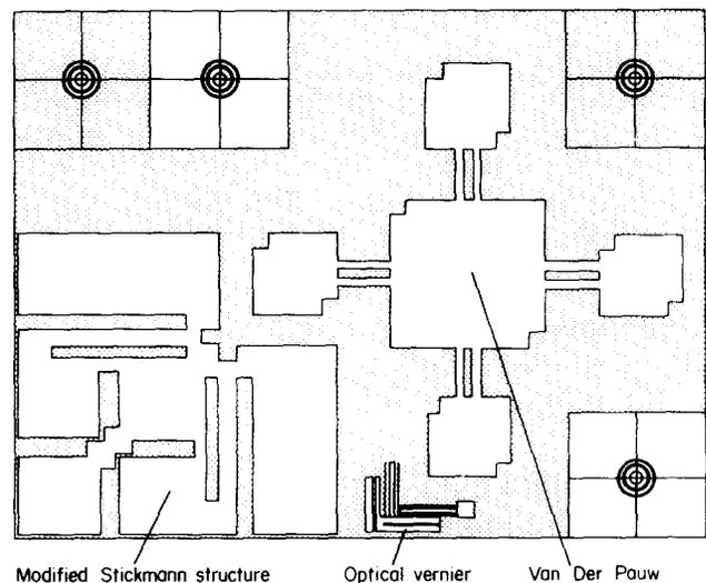
Fig 4 Unit cell electrical registration structure
