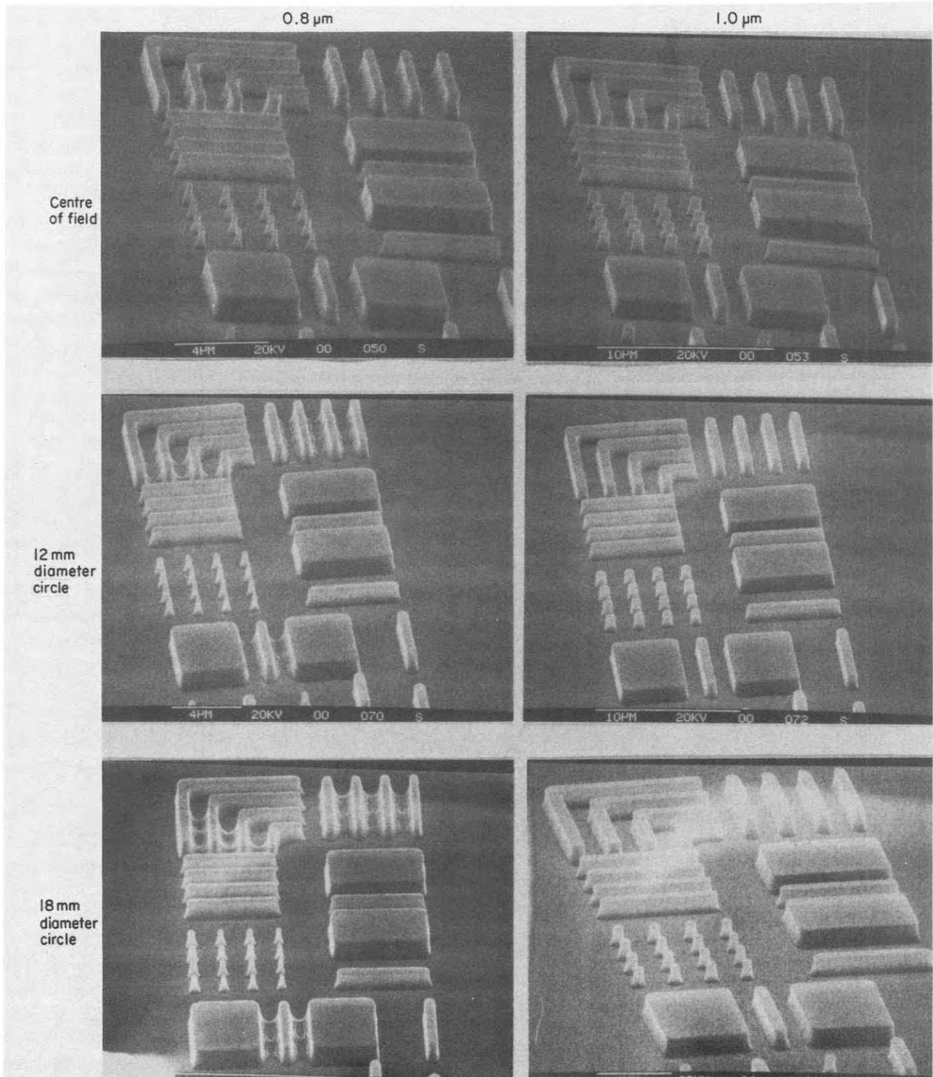
Fig 1 Cross-frame resolution, optimized photoresist process
