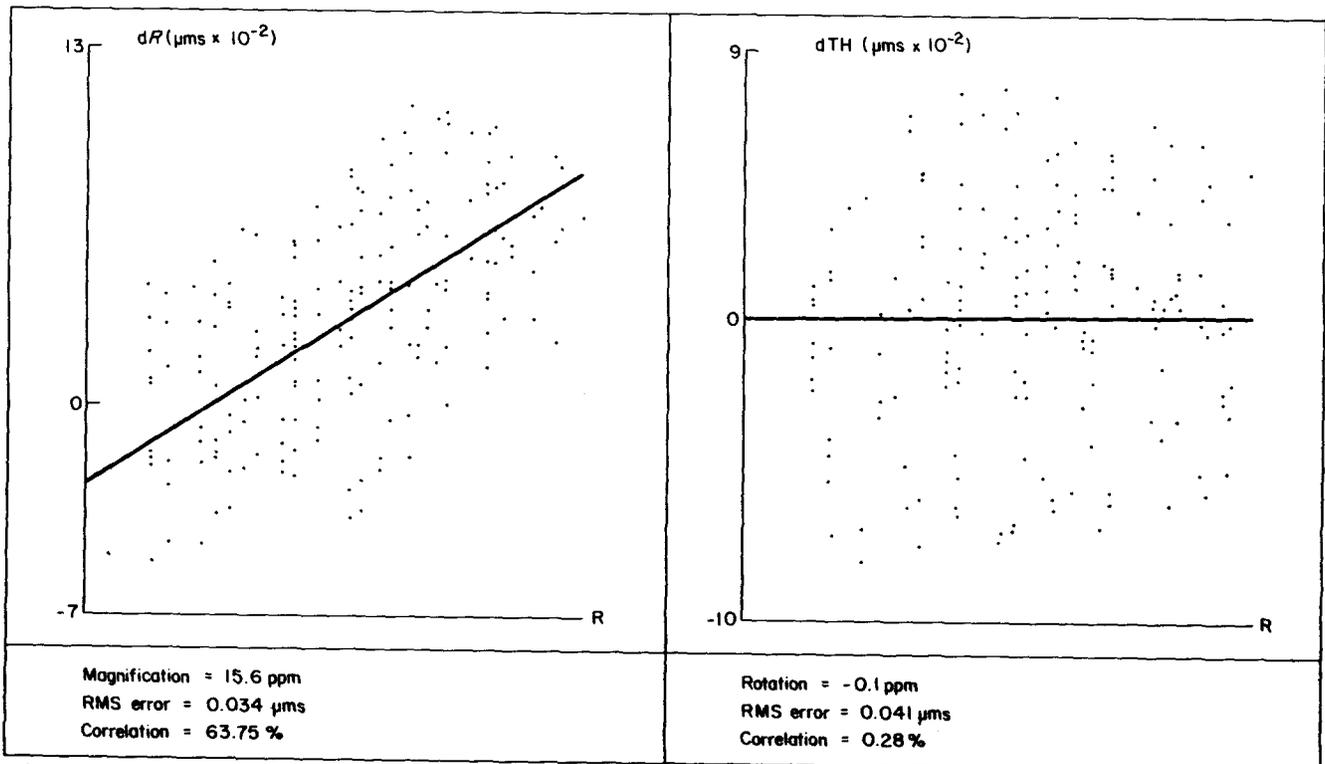
Fig 8 Polar errors showing rotation and reduction
