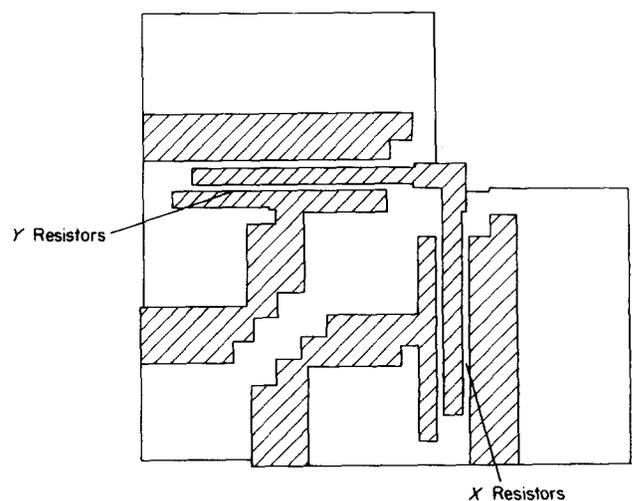
Fig 5 Overlaid registration structure. (The shaded areas are not a feature)
