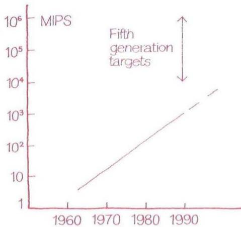
In the past, system performance has increased regularly by a factor of ten each decade. This improvement has been achieved by advances in circuit technology and by increasingly complex systems. For the future, VLSI offers the potential of much greater circuit complexity but only modest increases in circuit performance.
