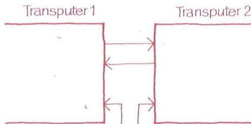
The IMS T424 has four standard INMOS links providing high speed intercommunication between transputer products, enabling a rich variety of networks to be constructed. Each link operates independently, and provides a memory to memory message (block) transfer capability between transputers.
