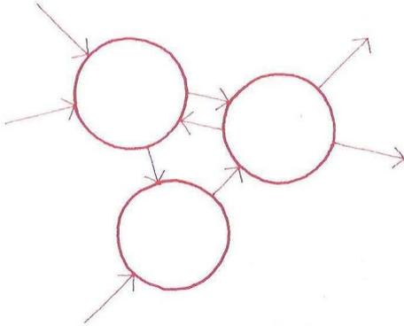
Processes can be connected together by channels to build more complex concurrent systems
