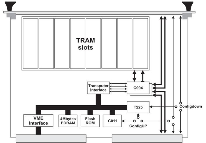
The TMB14 and TMB15 are both 6U VME bus interface boards with 8 TRAM slots. Device drivers to interface the boards to Solaris 1.x and Solaris 2.x running on a Force 3CE SPARC based board are available.
