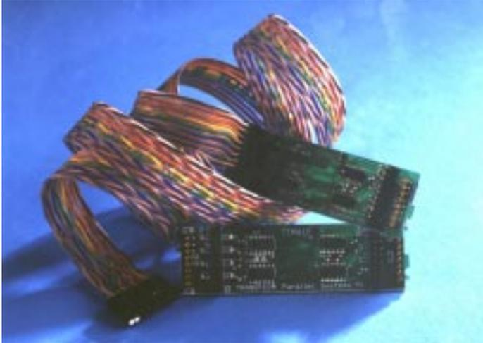
The TTM415 Differential Interface Buffer TRAM allows connections between transputer systems which are not in the same electrical environment. No common ground between the two systems is required, reducing earthing problems. Cable lengths up to 10m can be operated at the full 20Mbits/s link speed. Longer cables up to 100m can be used at lower link speeds.
