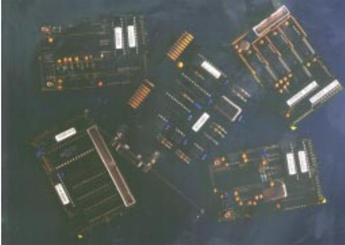
The range of Analog and Digital I/O TRAMs available are all compatible with Transtech's TRAM motherboards. Included in the range are 5 analog input modules, 2 digital to analog converter modules and 4 digital I/O modules.
