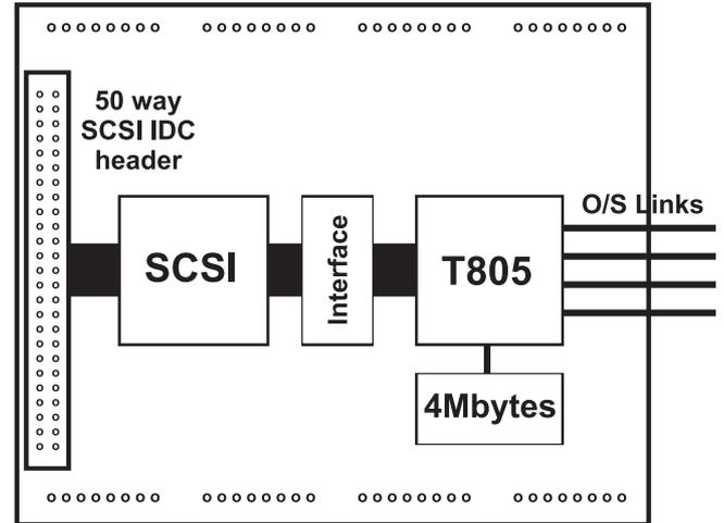
The Transtech TTM50 is a TRAM that provides a transputer to SCSI-2 interface. It is suitable for connecting a wide range of SCSI devices, including disks, tapes, CD-ROM and workstations to transputer networks.
