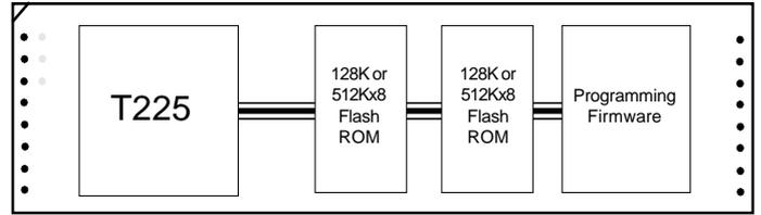
The TTM418 Flash ROM TRAM is designed primarily for configuring and bootstrapping transputer networks in embedded systems.
