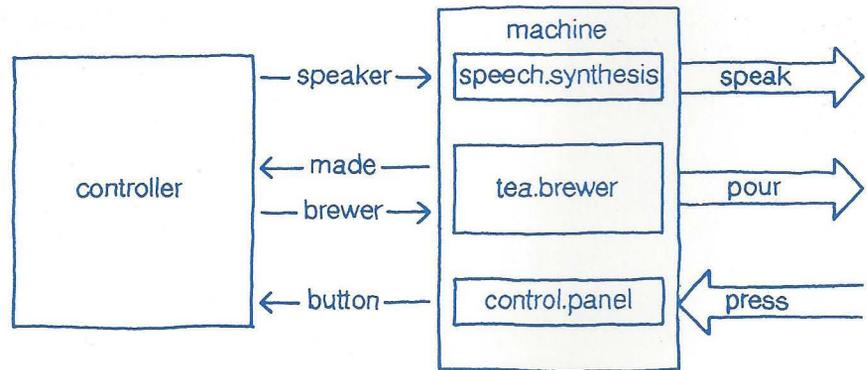
In occam, each of the units is described by a process and each connection by a channel. The processes communicate by sending messages via the channels. A process can be constructed from smaller processes, as in the case of this machine which has a number of parts. Indeed the collection of processes is itself a process in occam, and could be part of some larger system.
